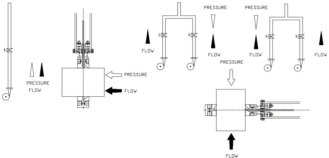
Special care should be taken to maintain the correct distance between the flanges and to ensure that they are parallel to the valve body. Incorrect alignment of the valve can cause deformations, which can lead to difficulties in operation.
