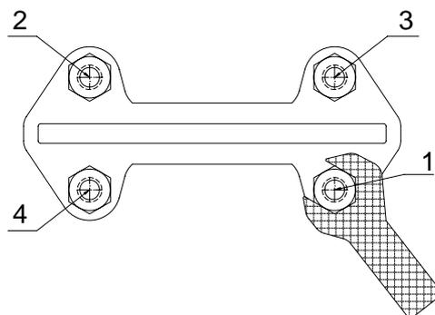
If the glandfollower nuts are pulled to hard, the force needed to operate the valve will increase, the valve function will be affected and the box packing lifetime will be shortened. The table below shows the maximum torque value for tightening the glandfollower nuts.
