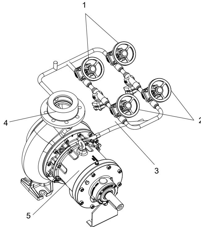
**Fig. 1:** Design of the circulation line
