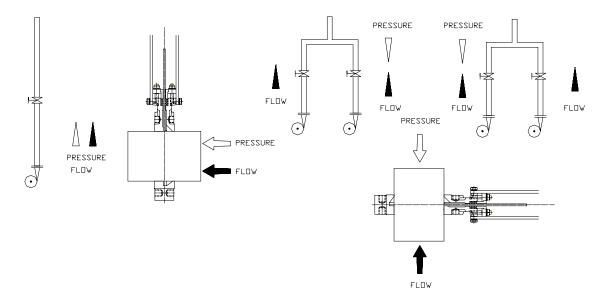
Special care should be taken to maintain the correct distance between the flanges and to ensure that they are parallel to the valve body. Incorrect alignment of the valve can cause deformations, which can lead to difficulties in operation.
