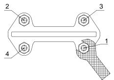
If the glandfollower nuts are pulled to hard, the force needed to operate the valve will increase, the valve function will be affected and the box packing lifetime will be shortened.
