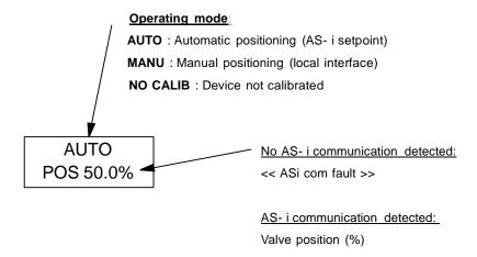
If the device has never been calibrated, the value of the position sensor in encoder steps is displayed (SSR).
