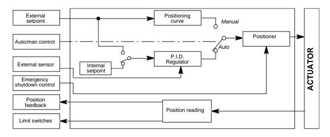
Positioning curve: setpoint position curve according to the external setpoint signal.
