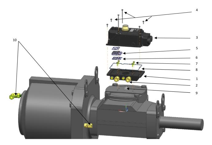
A – Check that the base (item 1) supplied with the unit is intended for this type of actuator. It must have two  $\frac{1}{4}$ " gas pneumatic openings (item 2 - connections not supplied) on the side, to supply the actuator chambers).
