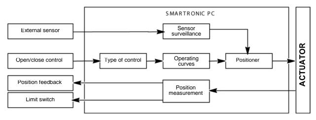
Sensor surveillance: definition of sensor values for which the valve moves to the safety position and an alarm is triggered. When this alarm is active, it takes priority over the open/close command.
