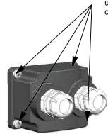
To access the electrical connection terminals unscrew the 4 TORX screws (T20) from the connection housing.
