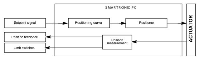
Positioning curve: position setpoint curve according to the external setpoint signal Positioner: automatically set by the self-calibration procedure.
