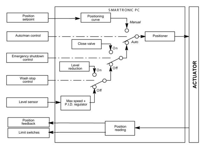
Positioning curve: setpoint position curve according to the external setpoint signal.
