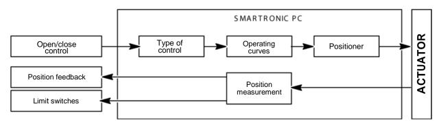
Type of control: normally open (control contact open  $\rightarrow$  valve open) or normally closed (control contact open  $\rightarrow$  valve closed) valve operation. Operating curves: valve open and close curves according to time. Positioner: automatically set by the self-calibration procedure.
