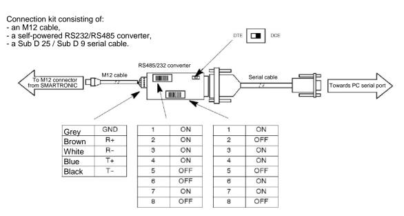
Make the connections according to the diagram above, checking the configuration of each of the switches on the converter.
