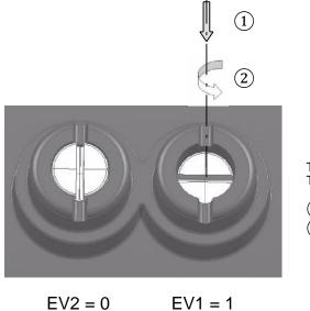
The emergency controls are fitted with a locking mechanism. To activate an emergency control:
