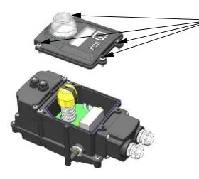
Unscrew the 4 TORX screws (T 20) in the cover. Tightening torque: 2Nm
