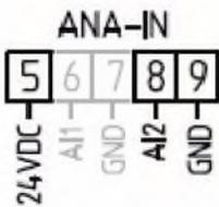
Input type: 4-20mA analogue input Input
