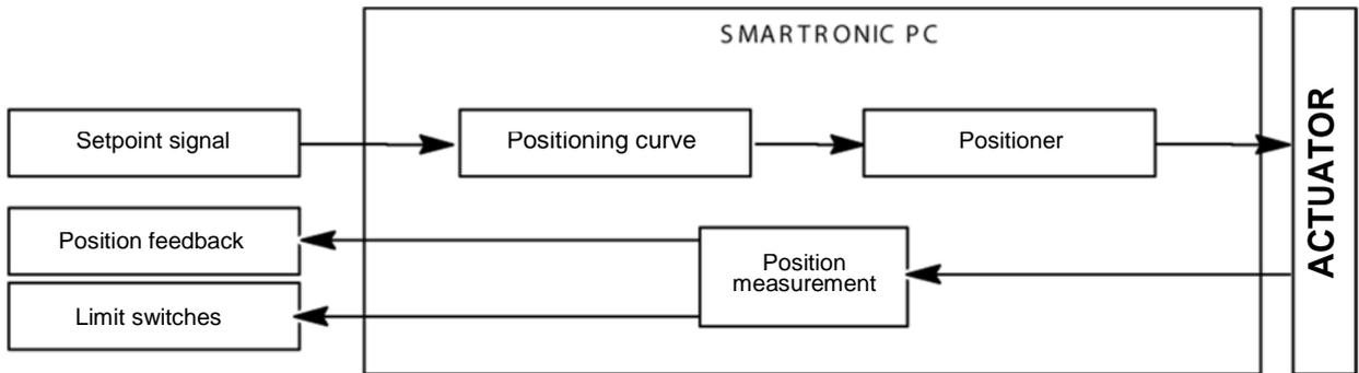
Positioning curve: position setpoint curve according to the external setpoint signal
