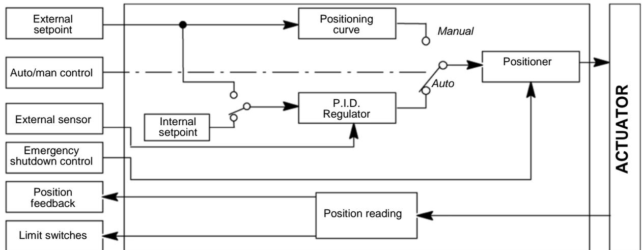
Positioning curve: setpoint position curve according to the external setpoint signal.
