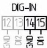
Input type: potential-free contact, power supply from the unit
