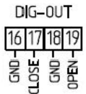
Output type: isolated outputs equivalent to dry contacts
