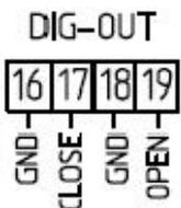
Output type: isolated outputs equivalent to dry contacts
