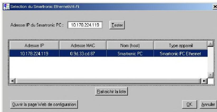
To modify the SMARTRONIC PC network parameters, in particular the name (host) in order to distinguish each SMARTRONIC PC, click the **Open configuration web page button**.
