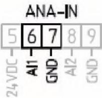
Input type: 4-20mA analogue input Input
