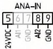
Input type: 4-20mA analogue input Input
