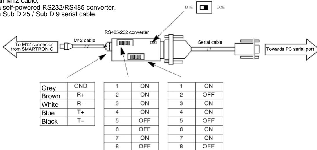
Make the connections according to the diagram above, checking the configuration of each of the switches on the converter.
