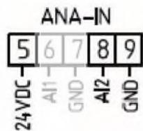
Input type: 4-20mA analogue input Input
