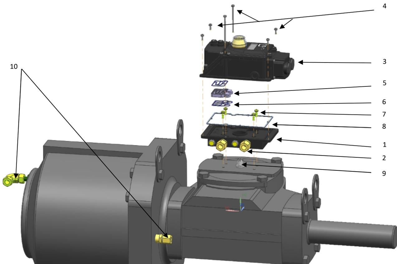
A – Check that the base (item 1) supplied with the unit is intended for this type of actuator. It must have two ¼" gas pneumatic openings (item 2 - connections not supplied) on the side, to supply the actuator chambers).
