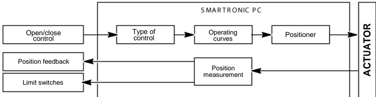
Type of control: normally open (control contact open → valve open) or normally closed (control contact open → valve closed) valve operation.
