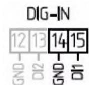
Input type: potential-free contact, power supply from the unit
