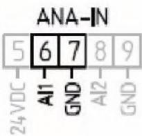
Input type: 4-20mA analogue input Input
