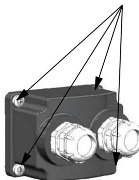
To access the electrical connection terminals unscrew the 4 TORX screws (T20) from the connection housing.
