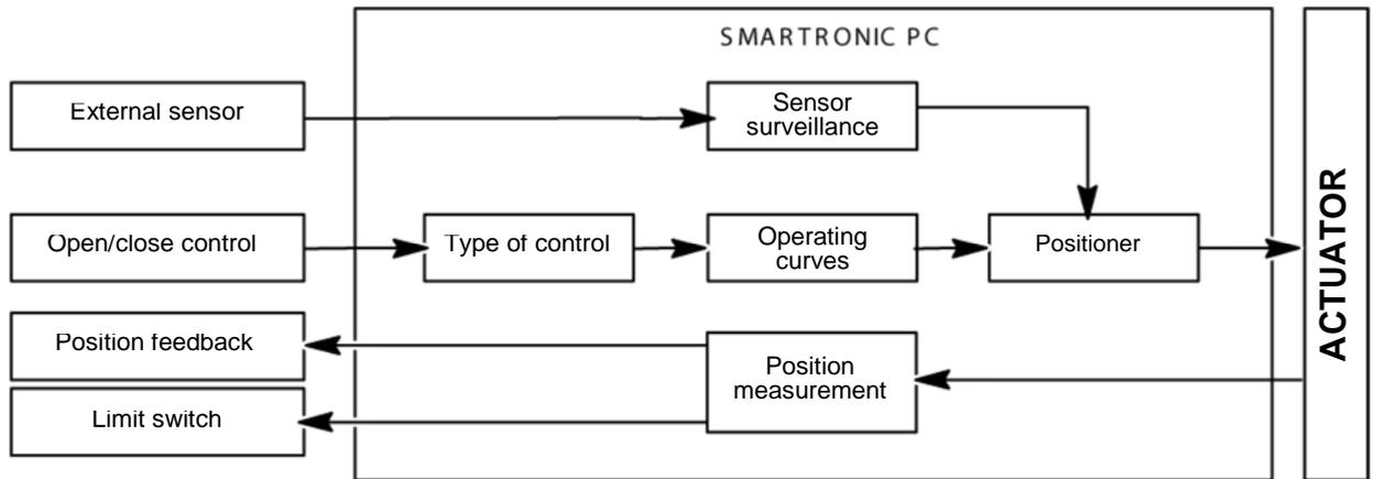
**Sensor surveillance:** definition of sensor values for which the valve moves to the safety position and an alarm is triggered. When this alarm is active, it takes priority over the open/close command.
