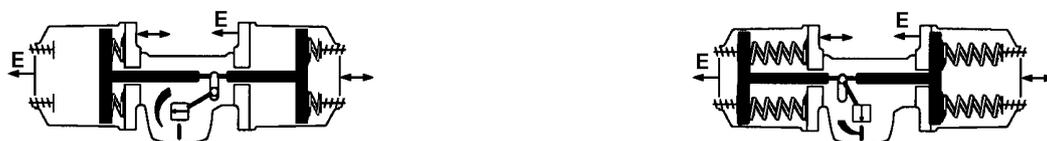
During the operation under pressure, the actuator is maintained in position by the air supply.
