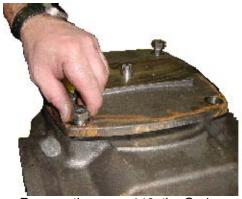
Remove the cover 142, the O-ring 412.5, the self-lubricating strip 310.2 and the O-ring 412.7
