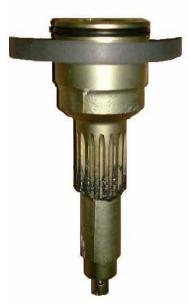
Position and at the same time, hold the lower bearing 300.2 on shaft 210 when inserting the scotch-yoke 59-26 with its index towards valve connection side
