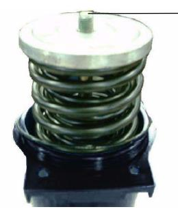
Smear on the ends adjustable of the stops 909 with Loctite glue (see paragraph consummable)
