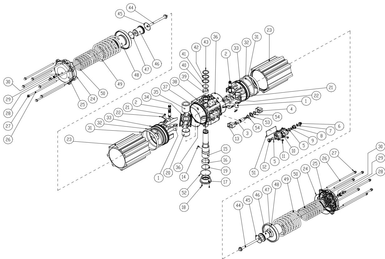
**Fig. 4:** Exploded view of size 260
