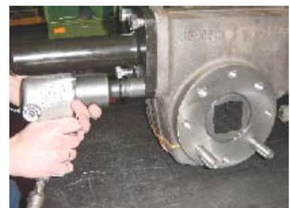
**REMOVAL OF PISTON 595 to be performed only if the stem seal 415 is damaged and/or defective**
