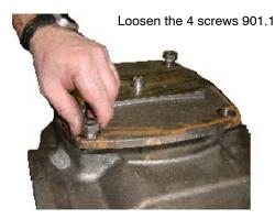
Remove the cap 142, O-ring 412.5, guide strip 310.2 and O-ring 412.7
