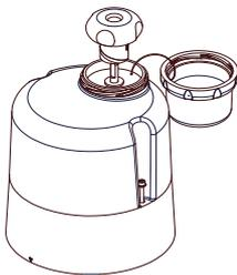
Fig. 10: Removing the protective cap of EA-C 140
