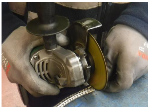
Fig. 20: Cutting the sealing cord
