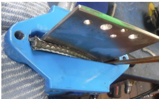
Fig. 22: Fitting the sealing cord
