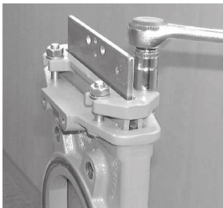
Fig. 14: Undoing the gland follower nuts
