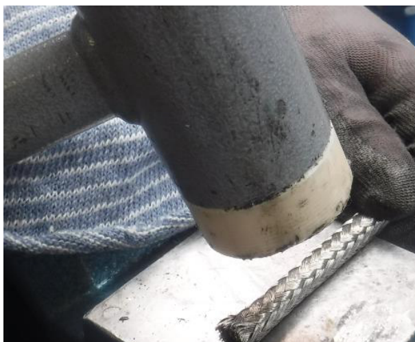
Fig. 21: Compressing the sealing cord
