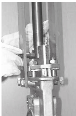
Fig. 13: Rising stem: Undoing the bolts
