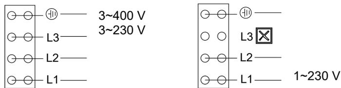
Fig. 5: Wiring diagram of automatic control unit to power supply
