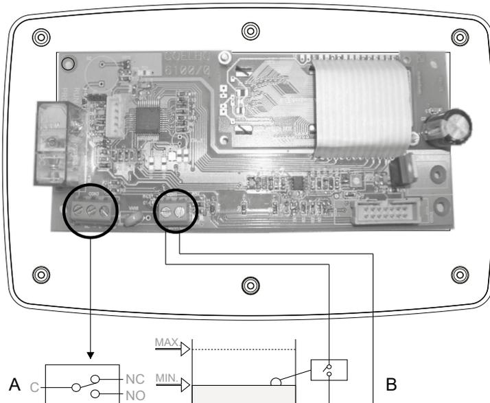
Fig. 6: Additional electrical connections
