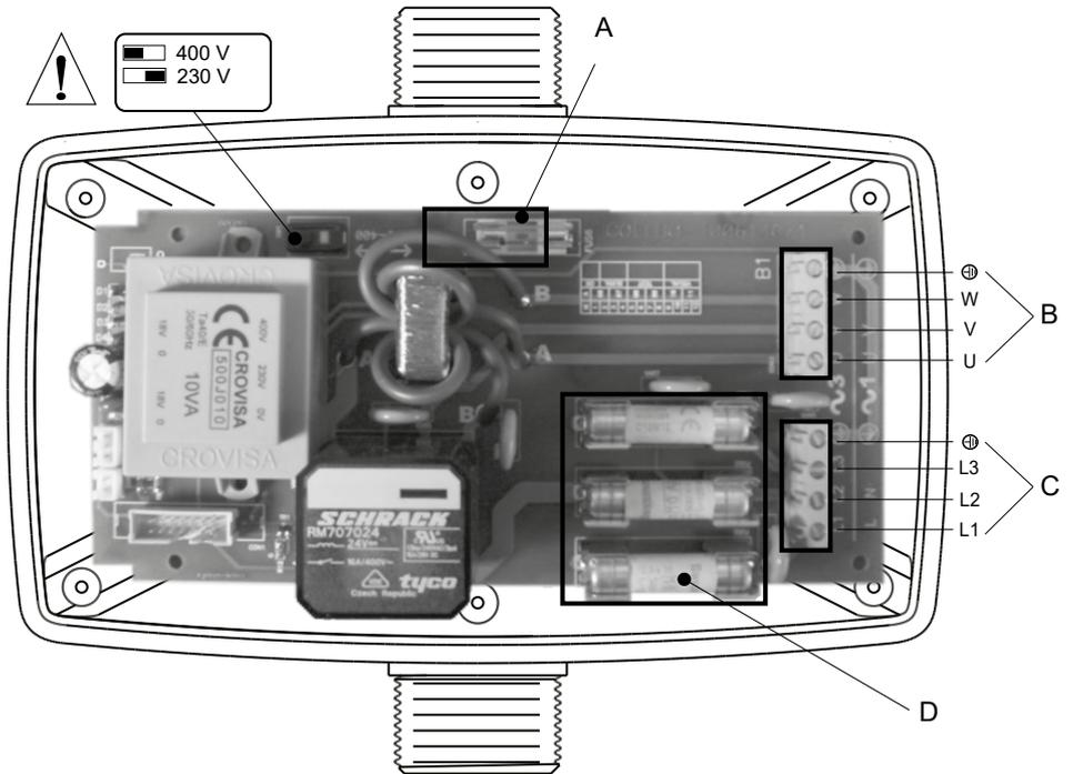
Fig. 3: Connections at automatic control unit
