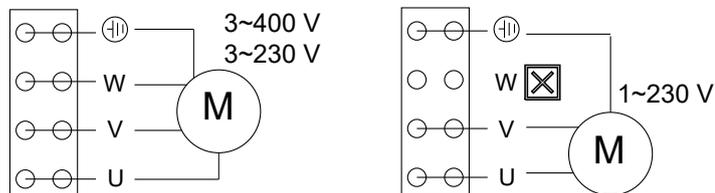
Fig. 4: Wiring diagram of automatic control unit to pump
