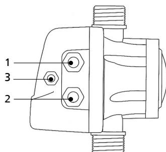
Fig. 7: Cable entry in housing
