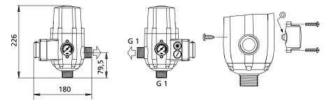
Fig. 4: Dimensions [mm] - The pressure gauge can be fitted in two different positions.
