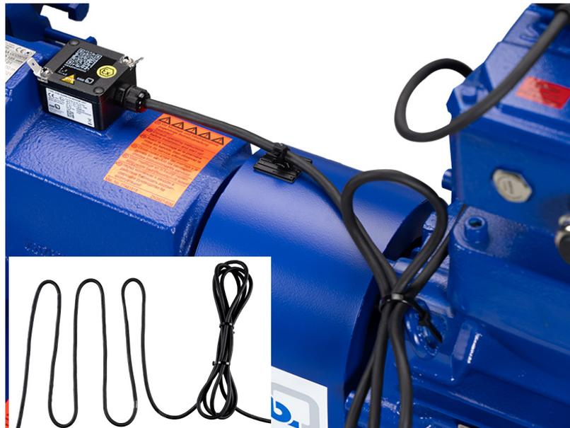
Fig. 14: Routing the connecting cable in a meander pattern
