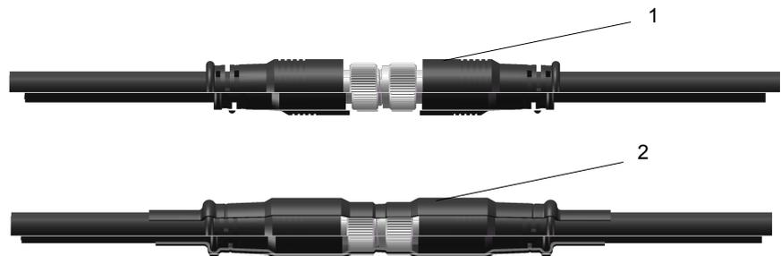
**Fig. 11:** Fitting the heat shrink tube
