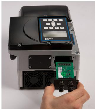
**Fig. 3:** Inserting the field bus module
