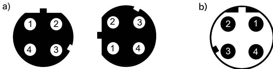
**Fig. 7:** Pin assignment: a) Module contact arrangement b) Connector contact arrangement
