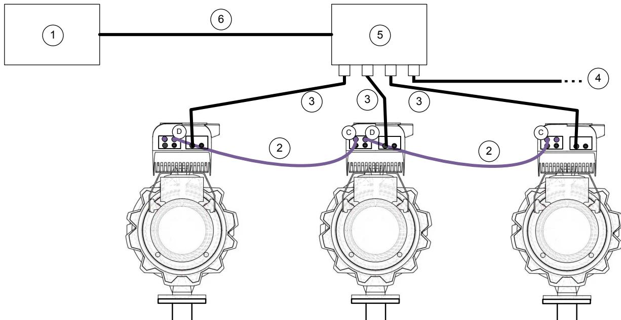
Fig. 10: Connecting the multiple pump system in the PROFINET network (example of star topology)
