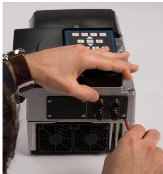
**Fig. 4:** Securing the field bus module
