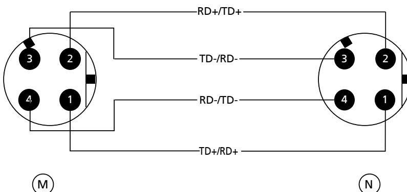
**Fig. 8:** User-configured cable for bus topology
