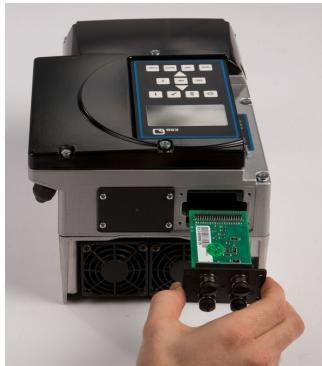
**Fig. 3:** Inserting the field bus module
