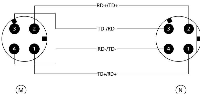
**Fig. 8:** User-configured cable for bus topology
