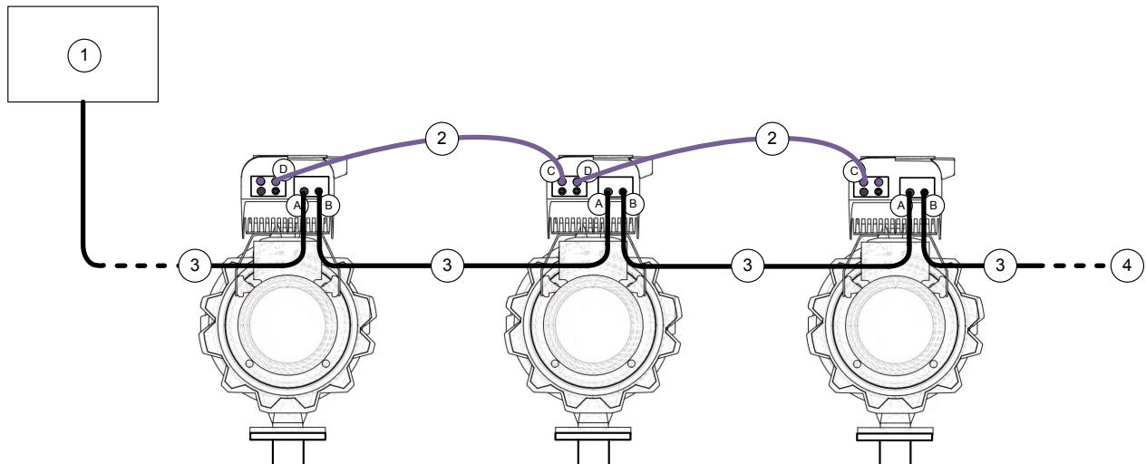
**Fig. 6:** Connecting the multiple pump system in the PROFINET network (example of bus topology)
