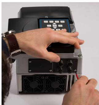
**Fig. 4:** Securing the field bus module
