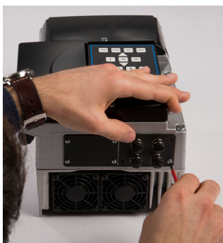
Fig. 4: Securing the field bus module
