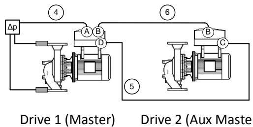
Special Firmware Modbus Master in PumpMeter is needed. In case of Etaline Z the special firmware is programmed in factory (DTM see also KSB Homepage)
