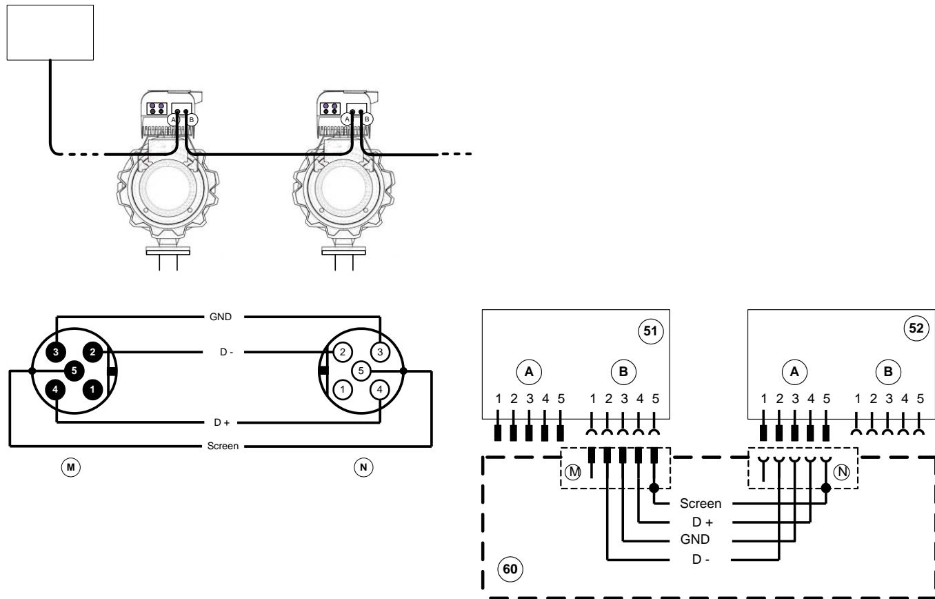
Self-made bus cable for fieldbus module BACnet:
