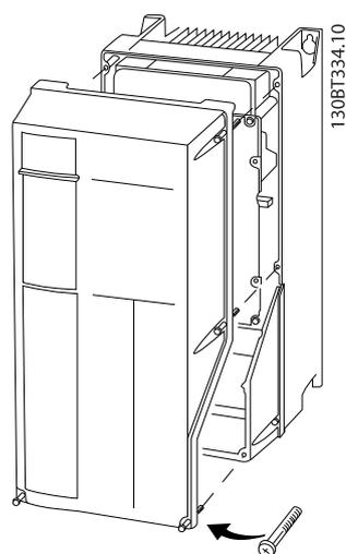
Illustration 4.4 Access to Wiring for IP55 and IP66 Enclosures
