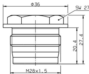
Fig. 20: Dimensions of the welding aid
