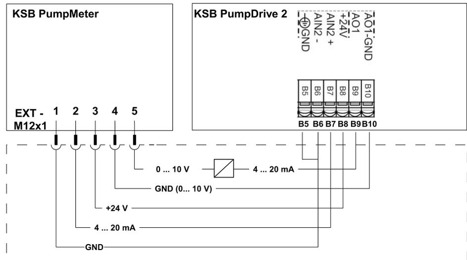
Fig. 14: Connection as differential pressure sensor via analog signal for pump operation with PumpDrive 2
