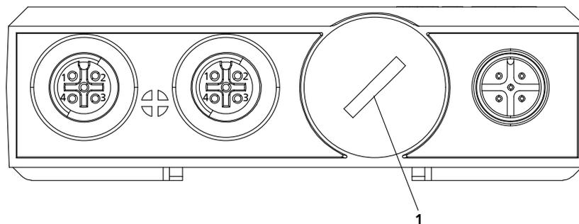
**Fig. 25:** Service interface connection
