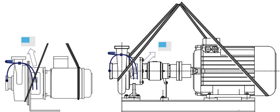
Fig. 2: Correct transport of device and pump (remove device)
