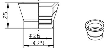
Fig. 19: Dimensions of the weld-in socket
