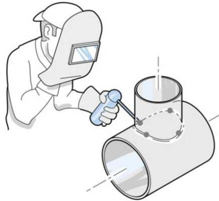
**Fig. 21:** Welding the weld-in socket into the piping
