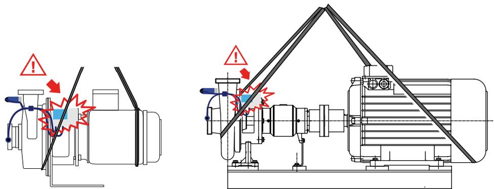
Fig. 1: Incorrect transport of device and pump
