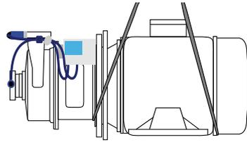
**Fig. 3:** Correct transport of device and pump (for  $\geq 5.5$  kW motors)
