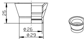
Fig. 19: Dimensions of the weld-in socket
