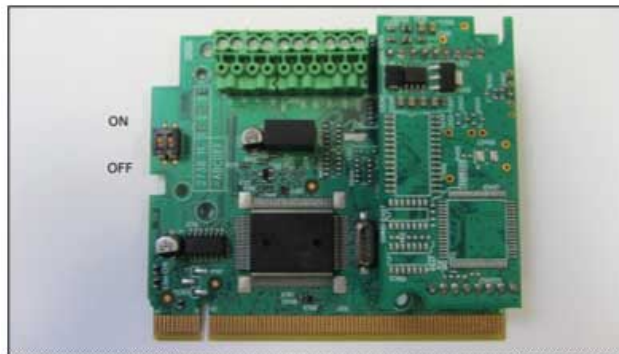
Fig. 1: DIP switches, terminating resistors
