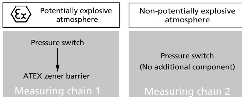
Fig. 26: Design of measuring chain
