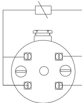
Fig. 6: Terminal assignment for PT100 four-wire system, pressure-proof (Ksb-4,13,xx,02)
