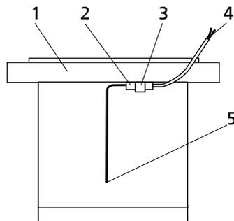
**Fig. 10:** Containment shroud with affixed mineral-insulated thermocouple
