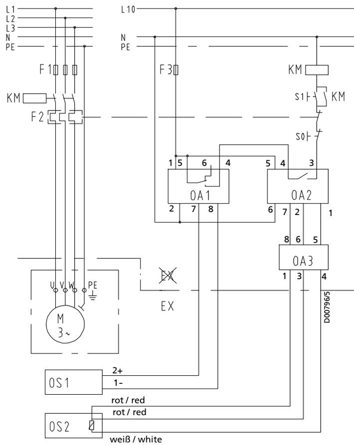
**Fig. 39:** Example of temperature monitoring at containment shroud with PT100 resistance thermometer
