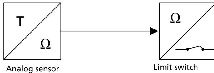
**Fig. 35:** Signal processing, analog sensor – limit switch using temperature monitoring as an example: intended operation
