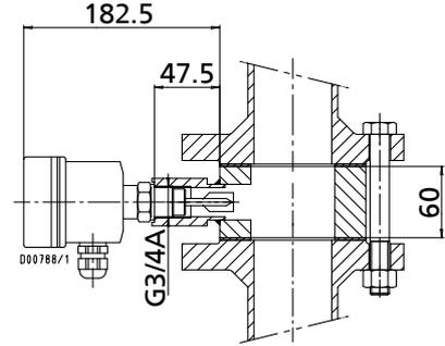
Installing the level transmitter with an intermediate piece in the pipeline
