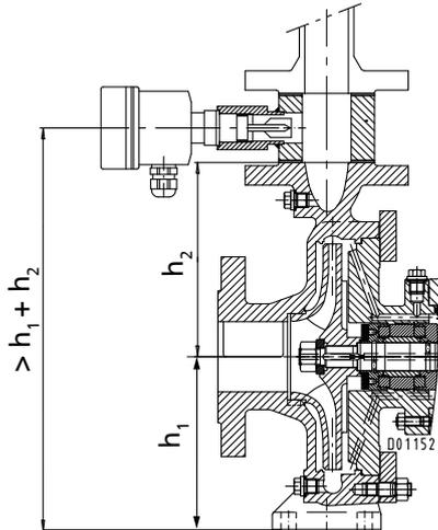
**Fig. 18:** Installing the level transmitter in the discharge line
