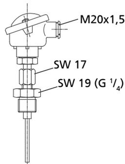
**Fig. 2:** PT100 resistance thermometer (Ksb-4,13,xx,02)
