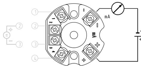
**Fig. 13:** Terminal assignment, mineral-insulated thermocouple with head transmitter
