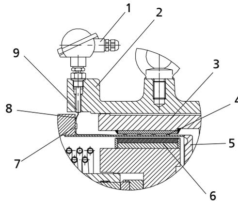
**Fig. 11: Fitting the mineral-insulated thermocouple**
