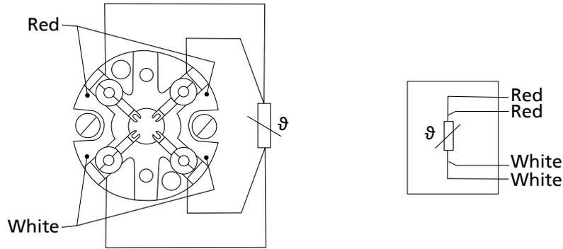
Fig. 5: Terminal assignment, four-wire system for TR 55
