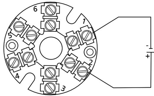
**Fig. 12:** Terminal assignment, mineral-insulated thermocouple with ceramic terminal block
