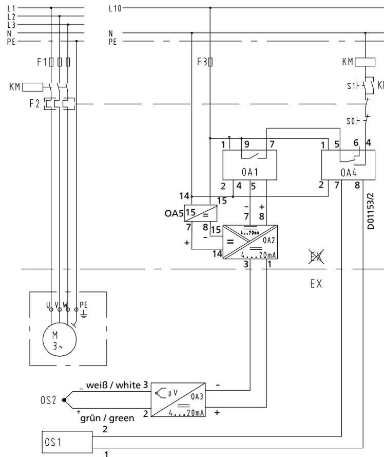
**Fig. 40:** Example of temperature monitoring at the containment shroud via a mineral-insulated thermocouple
