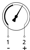
**Fig. 29:** Terminal assignment, contact pressure gauge
