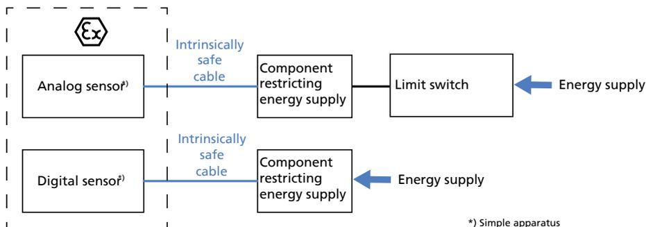
**Fig. 38:** Schematic representation of measuring chain
