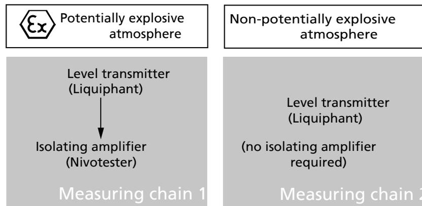
**Fig. 20:** Design of measuring chain
