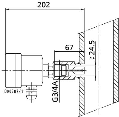
Installing the level transmitter with a weld-in socket in the pipeline
