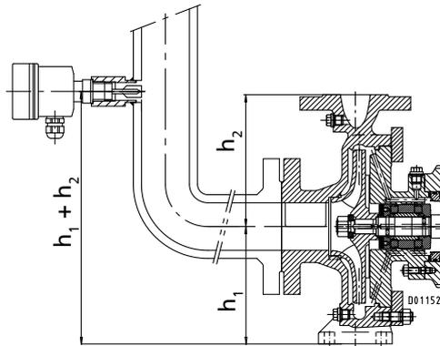
Fig. 17: Installing the level transmitter in the suction line
