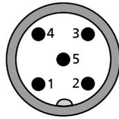
Fig. 25: Pressure switch terminal assignment
