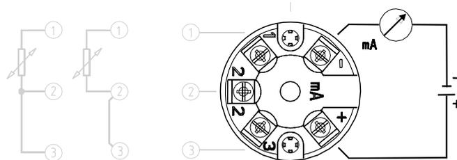
Fig. 7: Terminal assignment for PT100 including head transmitter (Ksb-4,13,xx,01 with T24)
