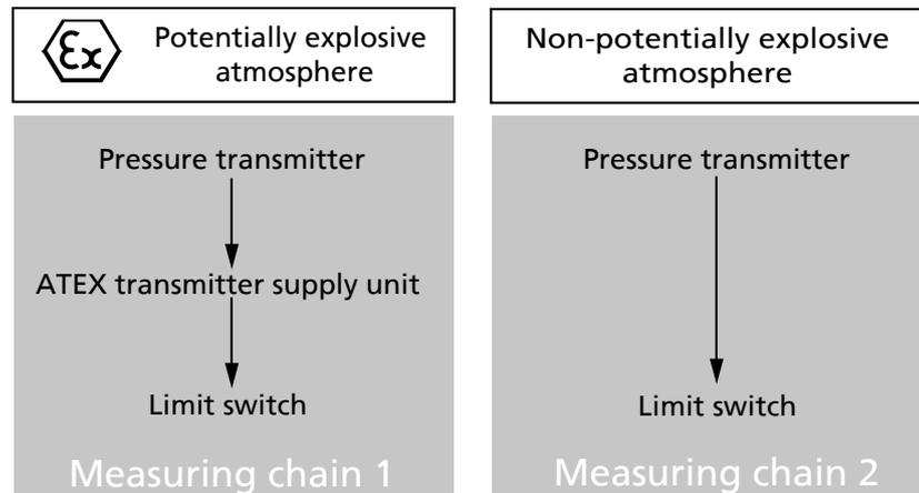
**Fig. 34:** Design of measuring chain
