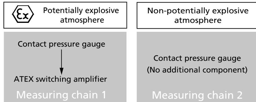
Fig. 30: Design of measuring chain
