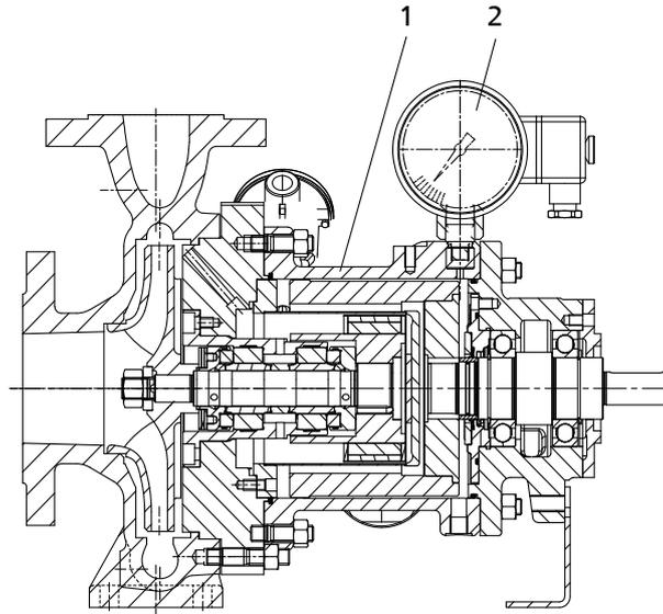
**Fig. 28:** Installing the contact pressure gauge
