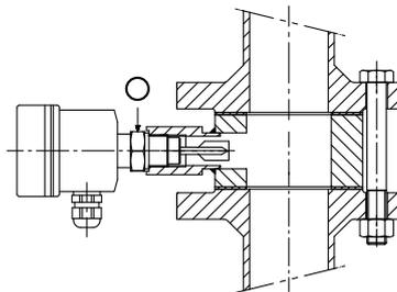
Fig. 16: Fitting level transmitter in pipeline
