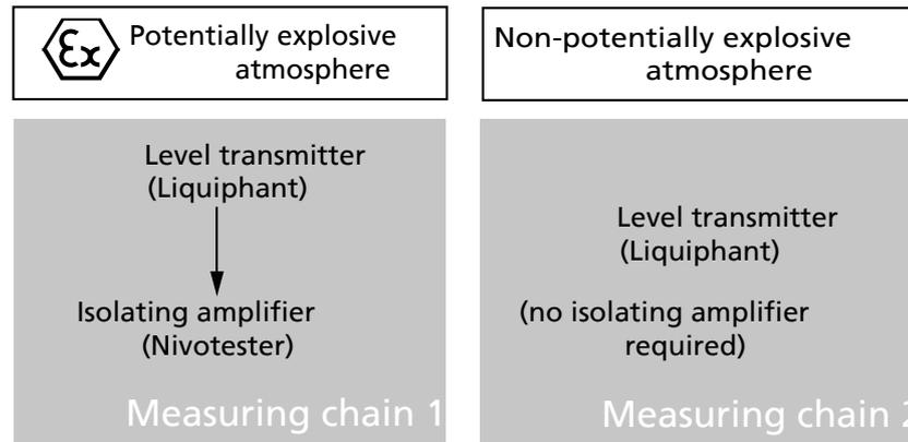
**Fig. 23:** Design of measuring chain
