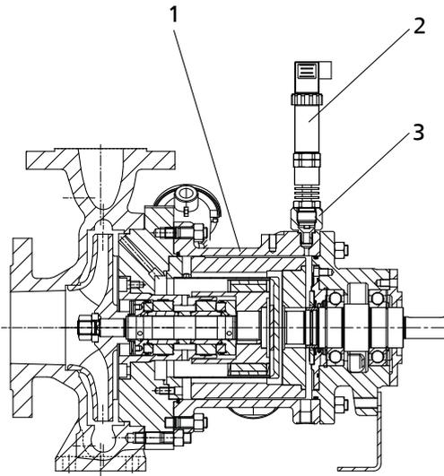
**Fig. 32:** Installing the pressure transmitter
