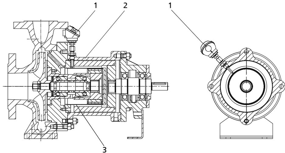
**Fig. 4:** Installation location of the PT100 resistance thermometer
