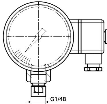
Fig. 27: Contact pressure gauge
