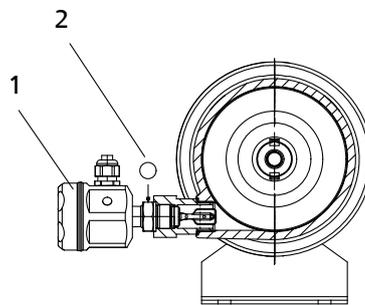
**Fig. 21:** Installing the level transmitter
