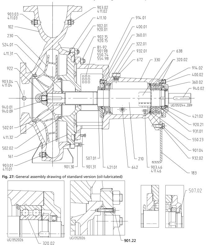
Version with clamped casing cover
