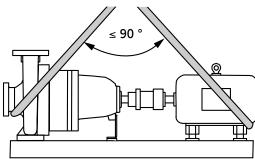
Fig. 3: Transporting the pump set
