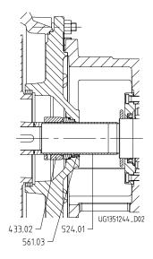
Mechanical seal with conical casing cover
