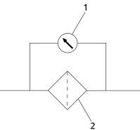
Fig. 9: Filter in the piping
