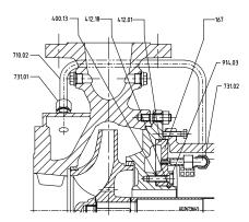
Heatable version with bolted casing cover
