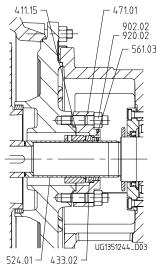
Mechanical seal with cylindrical casing cover
