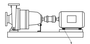
Fig. 17: Pump set with shim
