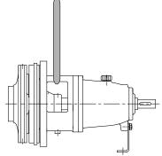
Fig. 1: Transporting the back pull-out unit
