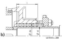
Fig. 22: Gland packing chamber a) with lantern ring and b) without lantern ring
