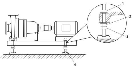
Fig. 8: Adjusting the levelling elements
