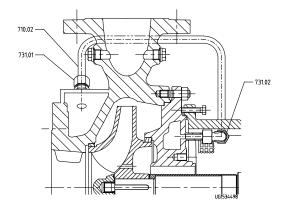
Heatable version with welded casing cover
