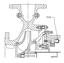
Heatable version, only casing cover cooled/heated
