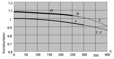
**Fig. 11:** Temperature correction diagram for "C, D, E, F, V, O variants" (1.4408 / A743 Gr. CF8M)
