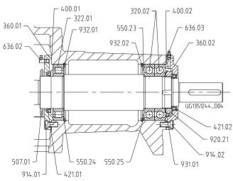
Grease-lubricated version (medium-duty bearing assembly)
