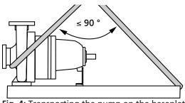
Fig. 4: Transporting the pump on the baseplate
