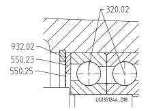
Fig. 21: Reassembling the medium-duty bearing assembly
