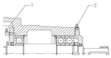
Fig. 20: Position of the lubrication nipples
