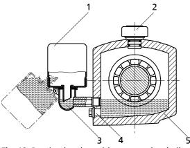
Fig. 18: Bearing bracket with constant level oiler
