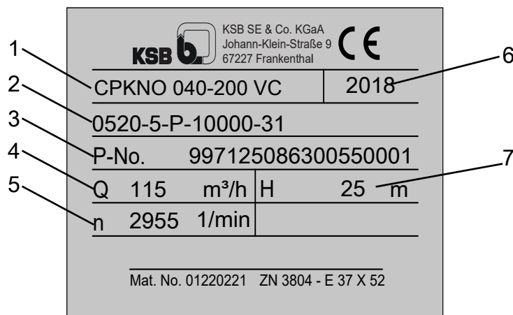
Fig. 5: Name plate (example)
