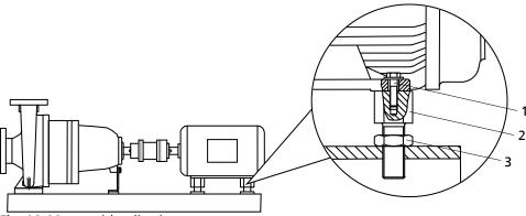
Fig. 14: Motor with adjusting screw
