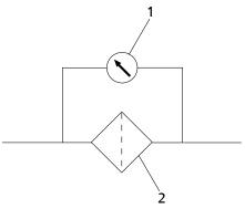
Fig. 9: Filter in the piping
