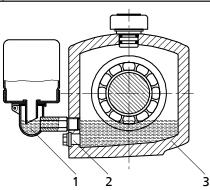
Fig. 17: Bearing bracket with constant level oiler
