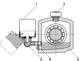
Fig. 16: Bearing bracket with constant level oiler
