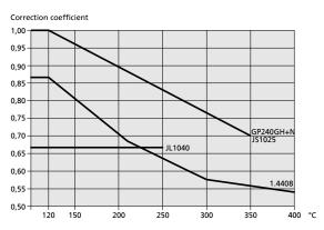
Fig. 10: Temperature correction diagram
