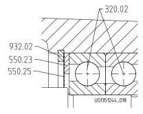
Fig. 19: Fitting the bearings
