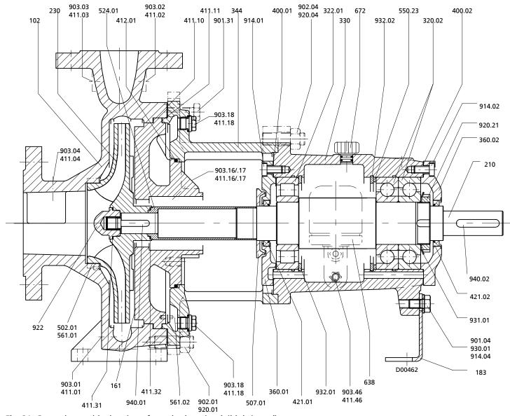
Fig. 21: General assembly drawing of standard version (oil-lubricated)
