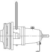
Fig. 1: Transporting the back pull-out unit
