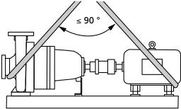
Fig. 3: Transporting the pump set
