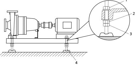
Fig. 8: Adjusting the levelling elements
