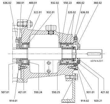
Fig. 23: Grease-lubricated version
