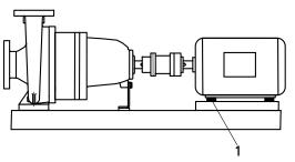
Fig. 15: Pump set with shim
