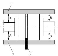
Fig. 11: Non-spacer-type coupling, checking the coupling alignment
