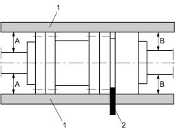
Fig. 12: Spacer-type coupling, checking the coupling alignment
