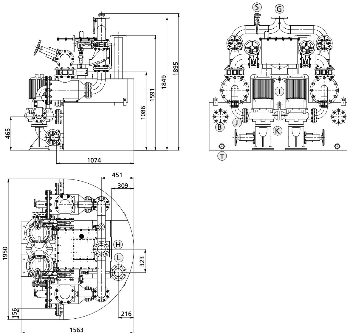
Dimensions, solids separation system (example) [mm]
