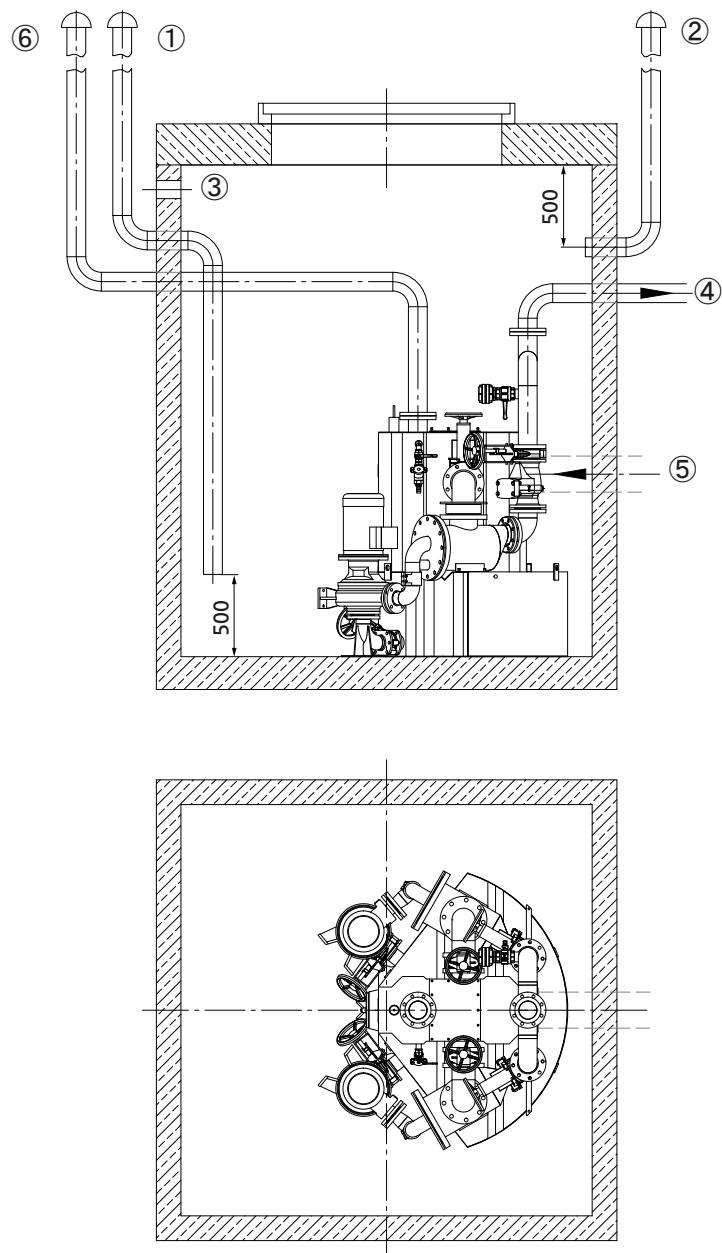
Installation example: angular concrete sump, dimensions specified in mm
