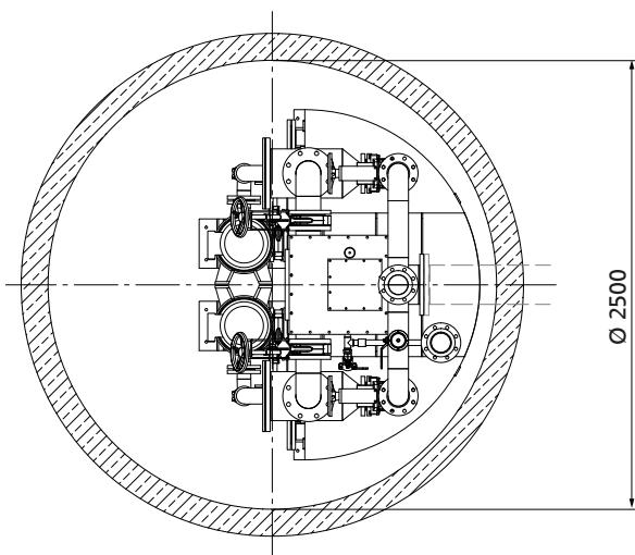
Installation example: circular concrete sump, dimensions specified in mm
