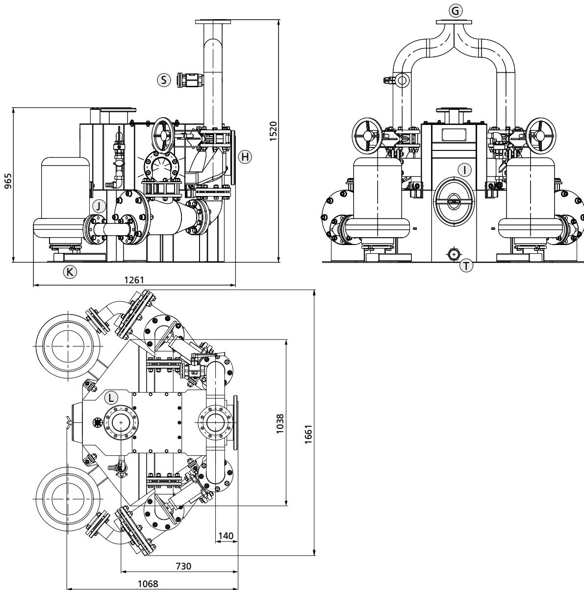
Dimensions, solids separation system (example) [mm]
