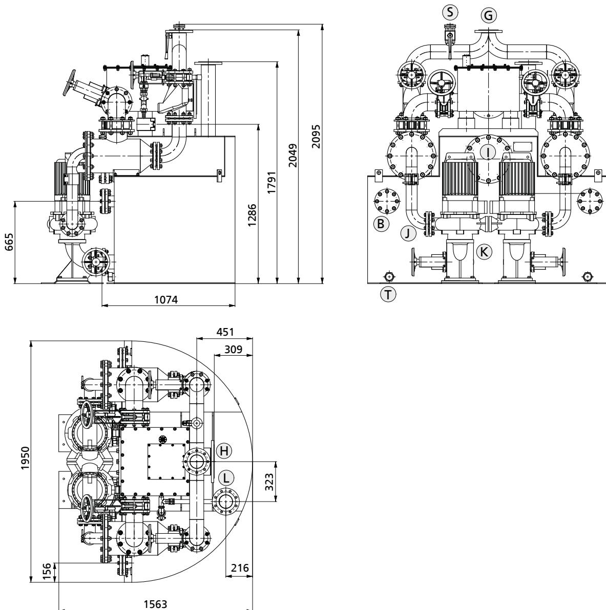
Dimensions, solids separation system (example) [mm]
