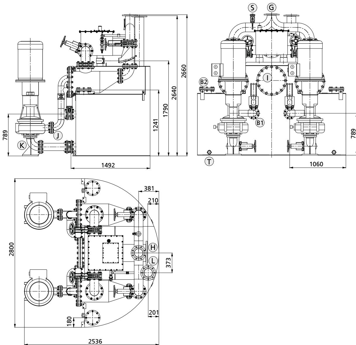
Dimensions, solids separation system (example) [mm]
