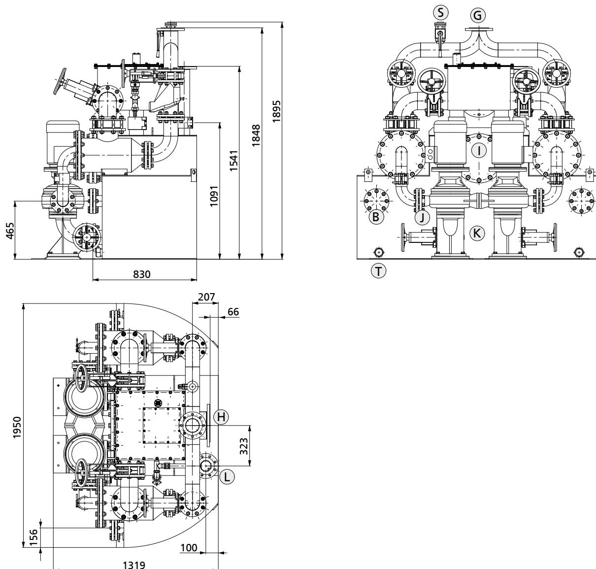
Dimensions, solids separation system (example) [mm]
