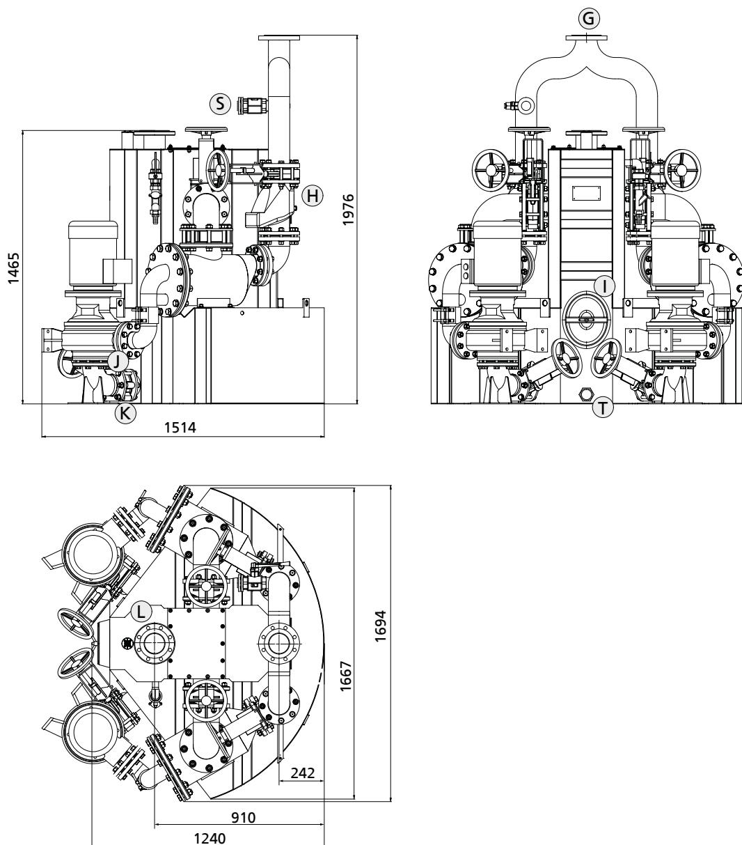
Dimensions, solids separation system (example) [mm]
