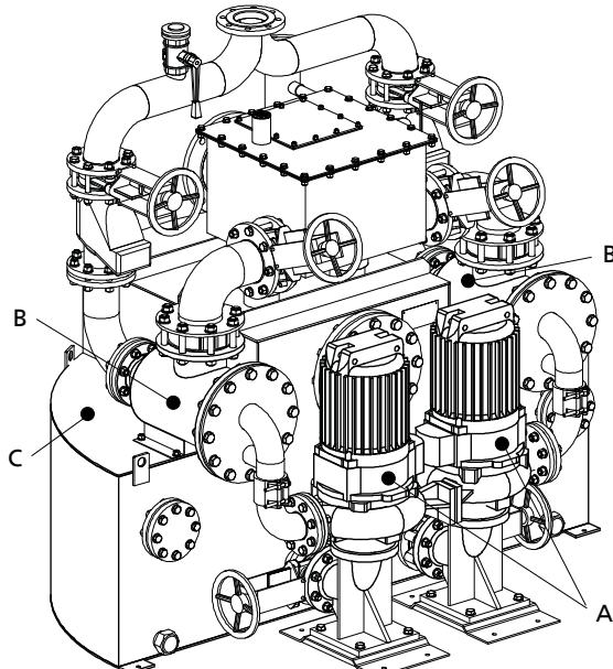
Design with semi-circular collecting tank
