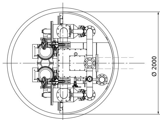
Installation example: polypropylene sump, dimensions specified in mm
