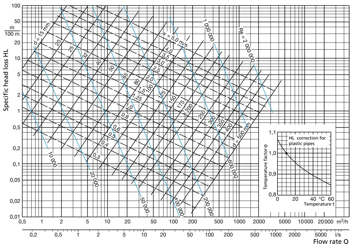
Head losses  $H_v$  for low-friction pipes ( $k = 0$ )
