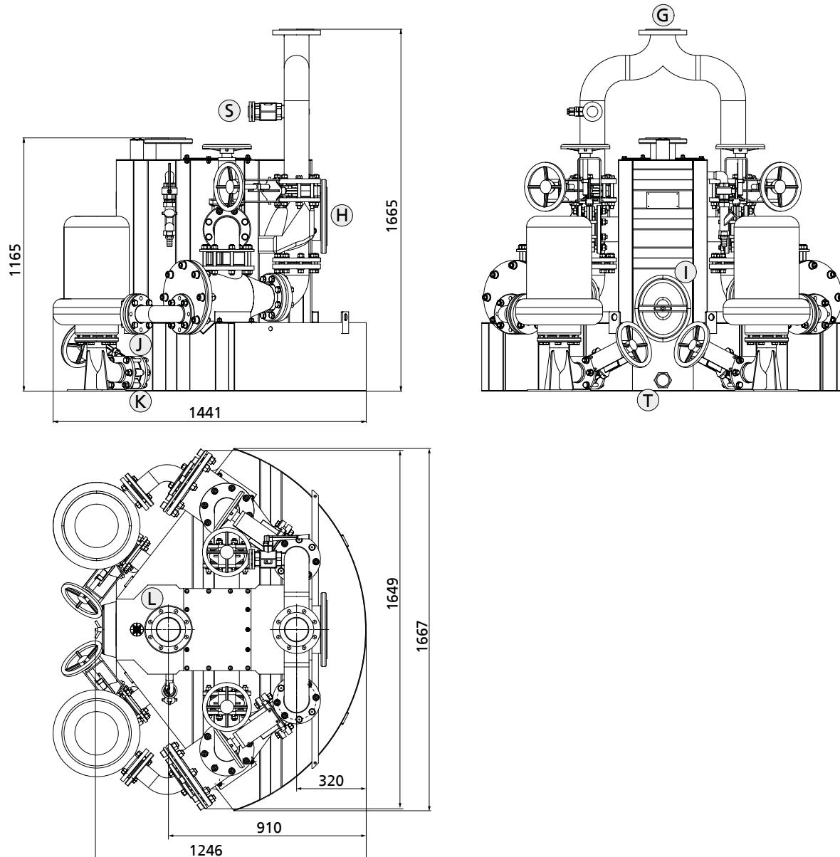
Dimensions, solids separation system (example) [mm]
