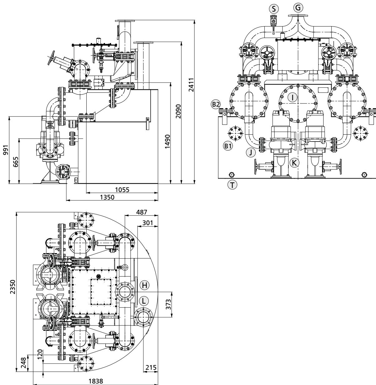
Dimensions, solids separation system (example) [mm]
