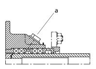
Uncooled gland packing with a) connection for barrier fluid or flushing liquid (connections 10 A.1 and 10 E.1)
