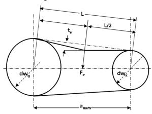
Fig. 18: Tension check for V-belts
