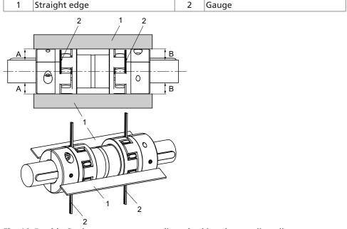
Fig. 16: Double Cardan spacer-type coupling, checking the coupling alignment
