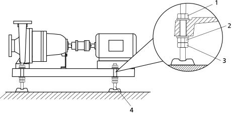
Fig. 11: Adjusting the levelling elements
