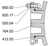
Fig. 22: Inspection hole in the casing
