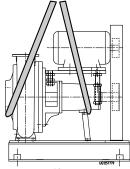
Fig. 3: Transporting a pump set with belt drive (figures 3Z and 4H)
