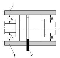
Fig. 14: Non-spacer-type coupling, checking the coupling alignment
