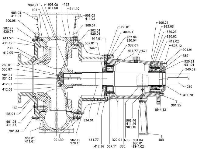
Fig. 29: General assembly drawing of pump with bearing bracket P10ax to P12sx: sizes 500-400-710 and 500-400-713
