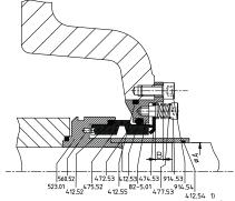
Fig. 32: 4K-120M mechanical seal<sup>39)</sup>
