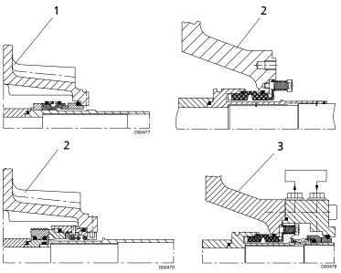
Fig. 8: Mechanical seals in conical seal chamber (A-type)
