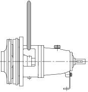
Fig. 1: Transporting the back pull-out unit
