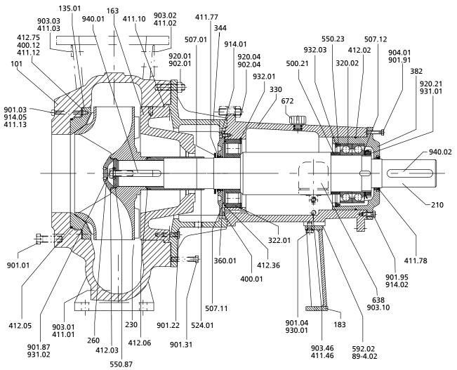
Fig. 28: General assembly drawing of pump with bearing bracket P08sx to P12sx
