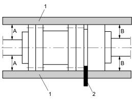
Fig. 15: Spacer-type coupling, checking the coupling alignment
