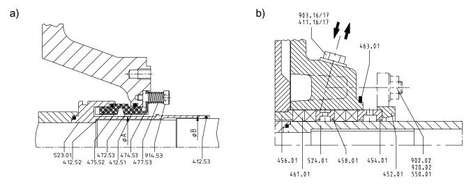
Fig. 31: Shaft seal P03ax to P12sx: a) 4K mechanical seal; b) coolable gland packing
