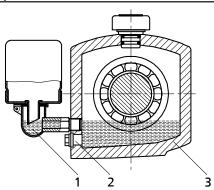
Fig. 23: Bearing bracket with constant level oiler
