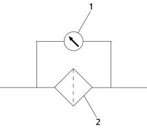
Fig. 12: Filter in the piping
