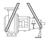
Fig. 2: Transporting the pump
