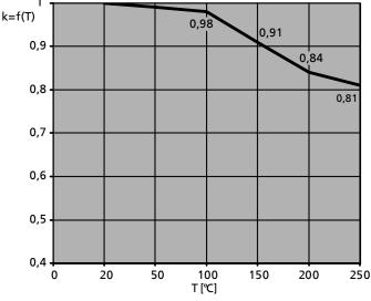
**Fig. 13:** Correction coefficient for material variant DDDD Calculation of forces and moments for T > 20 °C
