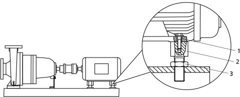
Fig. 19: Motor with adjusting screw
