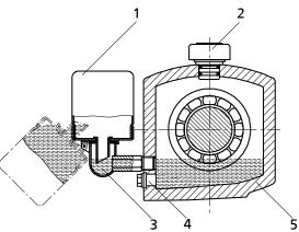
Fig. 21: Bearing bracket with constant level oiler
