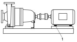
Fig. 20: Pump set with shim
