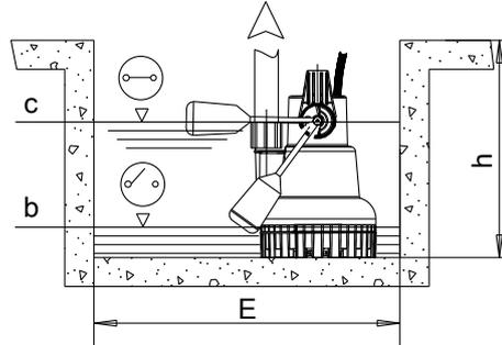
**Fig. 6:** Installation dimensions and switching levels
