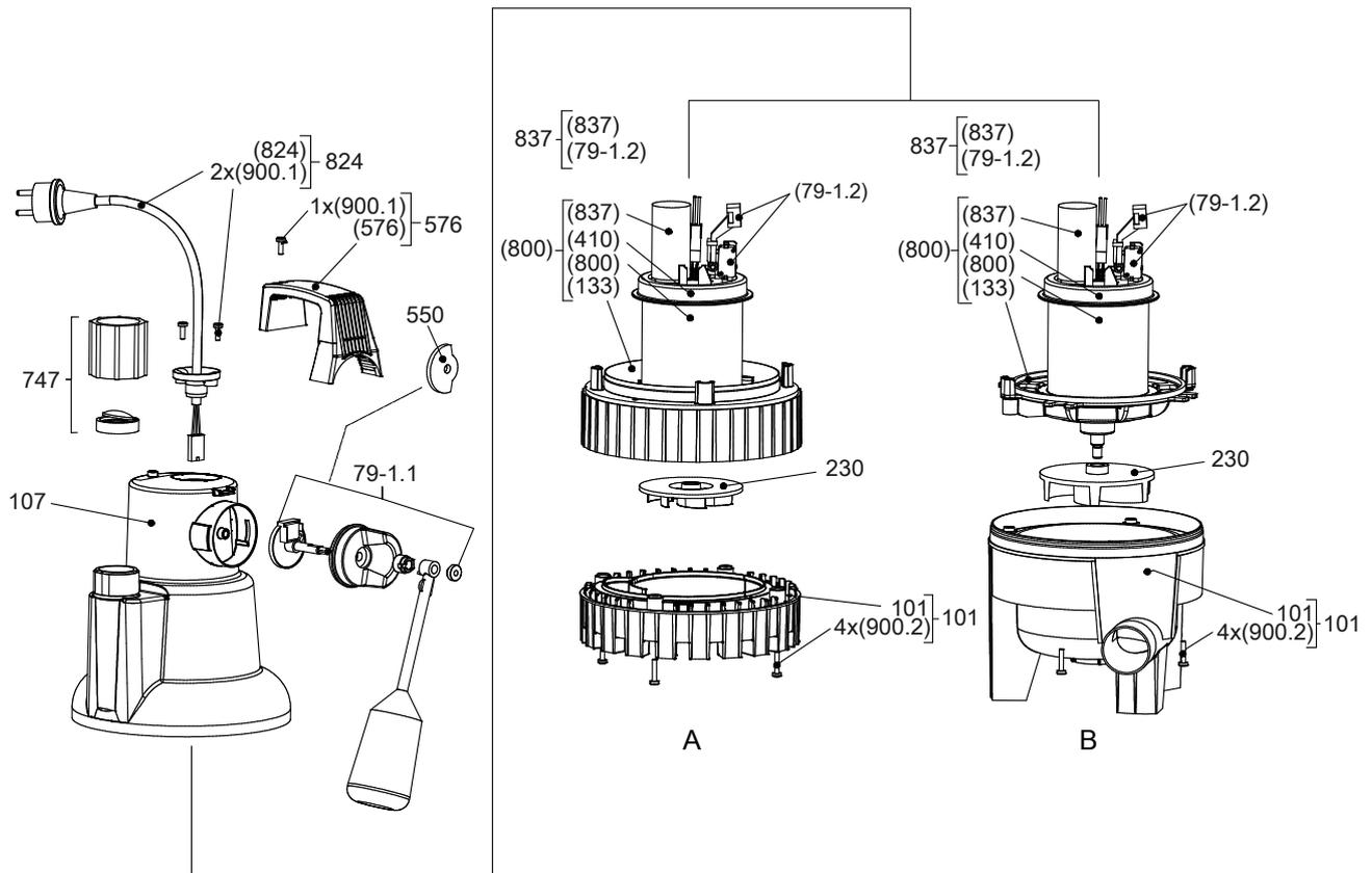
Fig. 11: Exploded view of Ama-Drainer N
