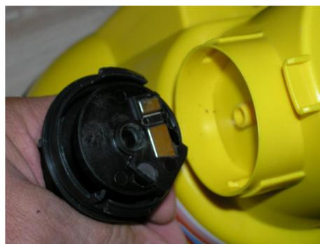
**Fig. 7:** Removing the automatic switchgear
