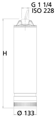
Abb. 1: Abmessungen Pumpenaggregat
