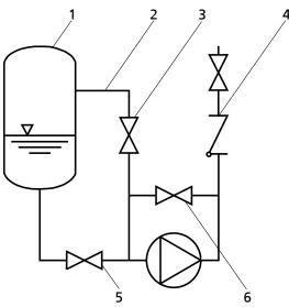
Fig. 8: Vacuum balance system
