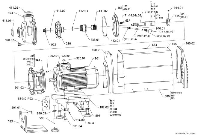
Fig. 12: Exploded view
