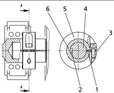
Fig. 6: Fitting the motor shaft stub on the shaft
