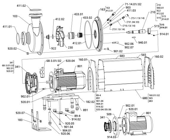
Fig. 13: Exploded view
