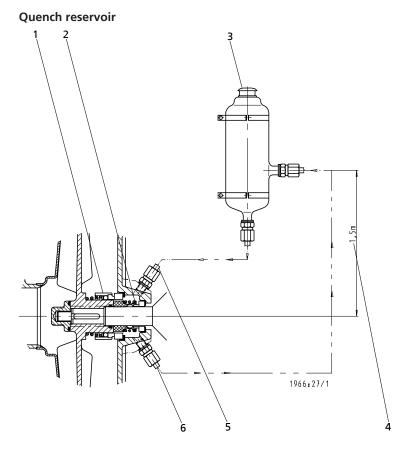
Fig. 22: Supply system with quench reservoir
