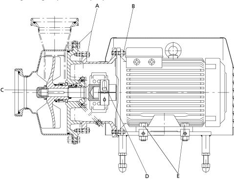
Fig. 10: Tightening points
