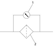
Fig. 7: Filter in the piping
