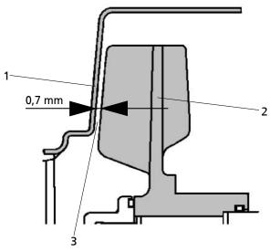
Fig. 9: Axial clearance between pump casing and impeller
