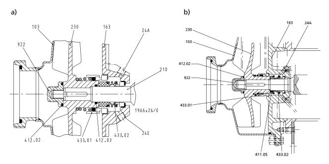
Fig. 20: Double mechanical seal a) with O-ring (size group I) b) with V-ring (size group II)
