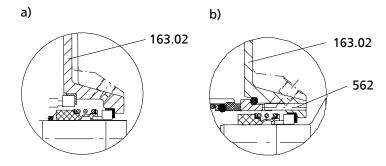
Fig. 21: Single or double mechanical seal a) without anti-rotation device, b) with anti-rotation device
