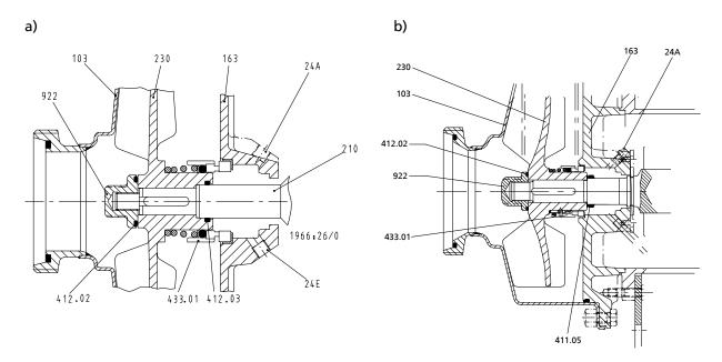
Fig. 19: Single mechanical seal a) with O-ring (size group I) b) with V-ring (size group II)
