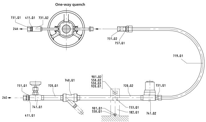
Fig. 23: Quench piping for one-way quench supply system
