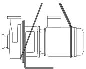
Fig. 2: Transporting the pump set (with angle foot, for motors  $\leq 4 \text{ kW}$ )
