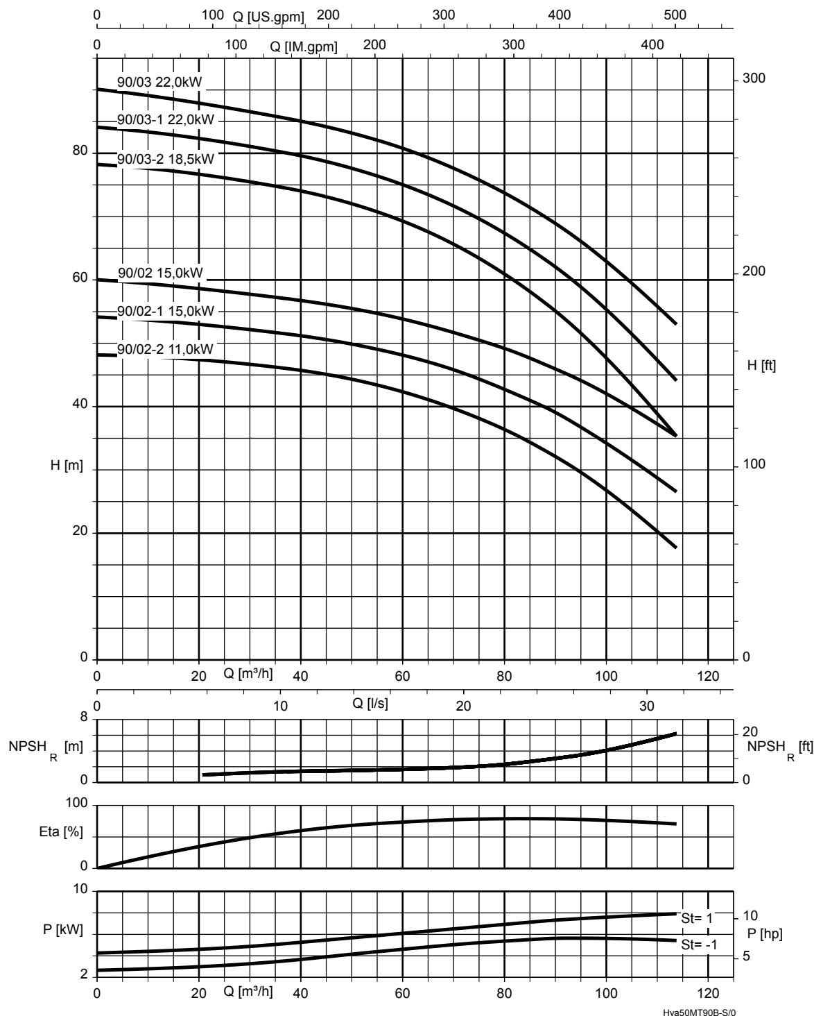
**Fig. 6:** Systems with 2, 3-2 and 3 stages
