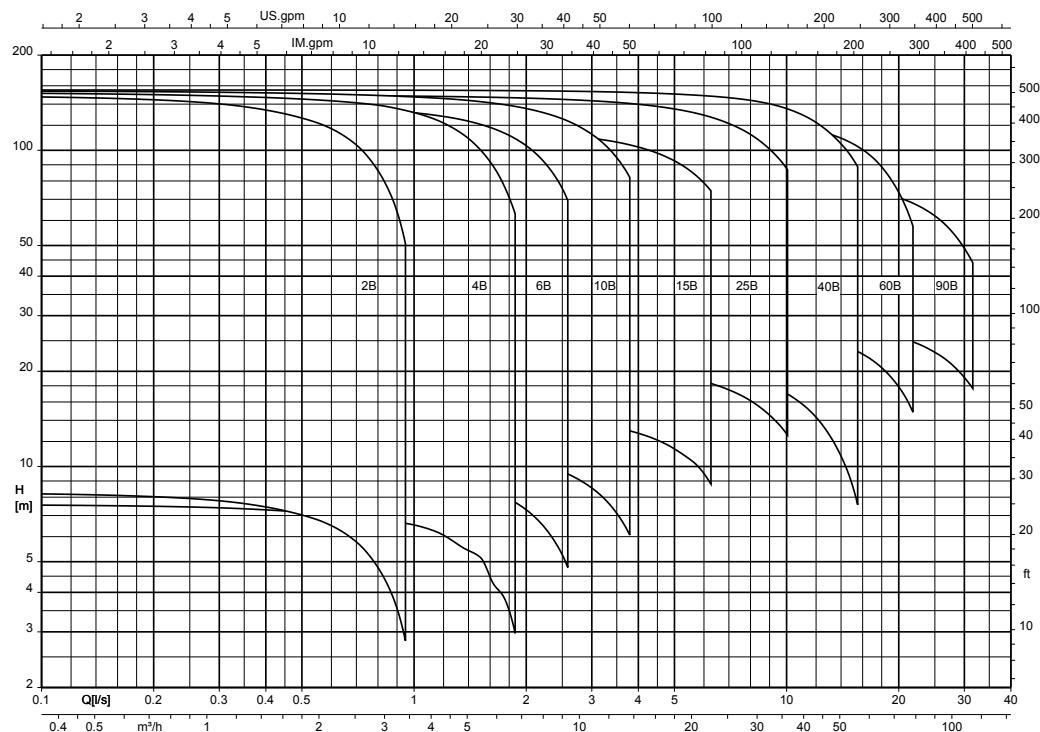
The flow rate in the characteristic curves is based on one duty pump:
