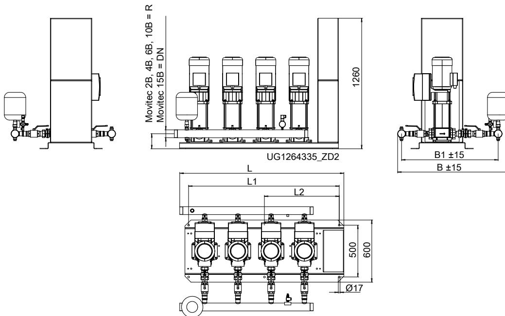
**Fig. 7:** Dimensions of version with Movitec 2B / 4B / 6B / 10B / 15B
