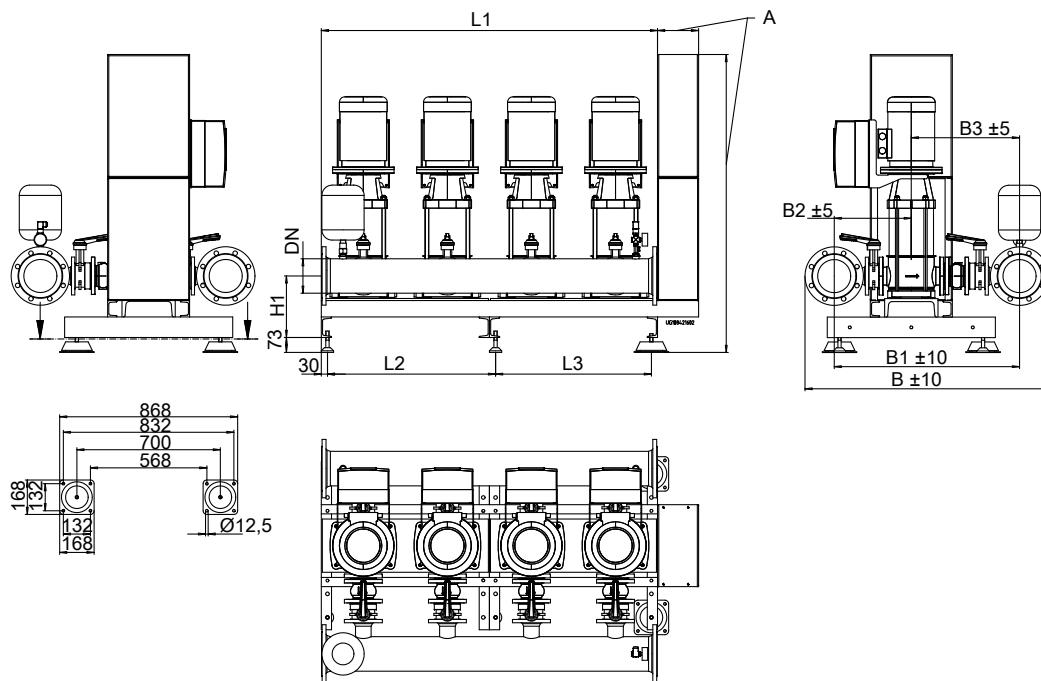
**Fig. 8:** Dimensions of version with Movitec 25B / 40B / 60B / 90B
