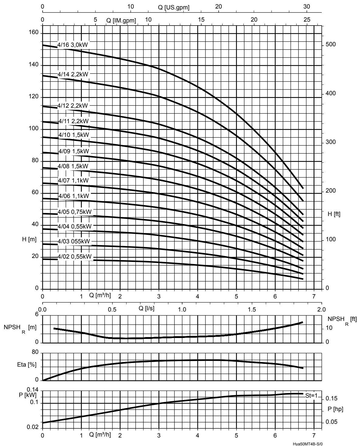
**Fig. 3:** Systems with 4, 5 and 10 stages
