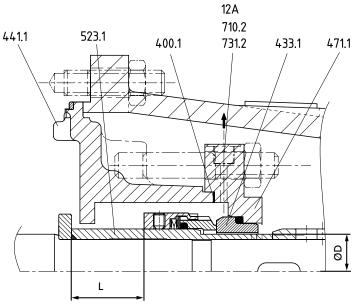
Fig. 46: Adjusting dimension L for mechanical seal
