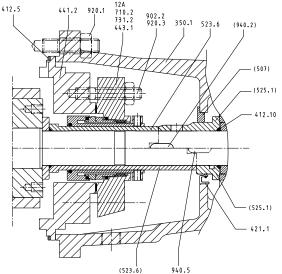
Fig. 39: Removing a cartridge seal
