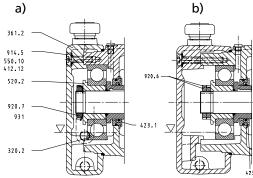
Fig. 30: Oil lubrication with labyrinth seal: a) Multitec 32-125 and b) Multitec 150-200
