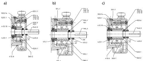
**Fig. 34:** Oil lubrication with labyrinth seal: a) size 32 and b) size 50-65 and c) size 100-200
