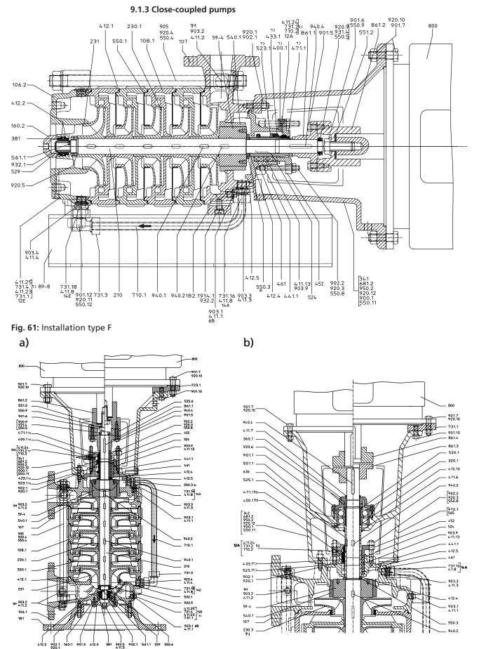
Fig. 62: Installation type V – a) size 32-65 – b) size 100-200
