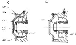
**Fig. 27:** Grease lubrication with labyrinth seal: a) Multitec 32-125 and b) Multitec 150-200
