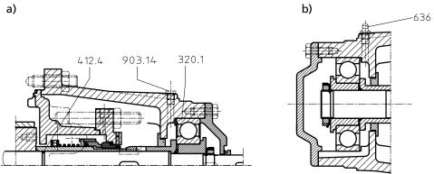
Fig. 64: a) Drive-end bearing on Multitec 32 - b) Grease lubrication with lubricating nipple, non-drive-end, sizes 100 and 125
