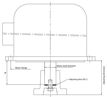
Adjusting dimensions for coupling alignment on sizes 32 to 65, installation types E, F, V,
