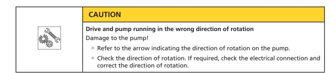
The correct direction of rotation of the motor and pump is clockwise (seen from the motor end).
