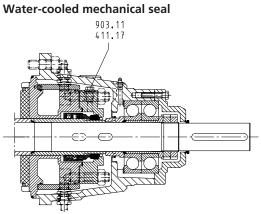
Fig. 11: Water-cooled mechanical seal
