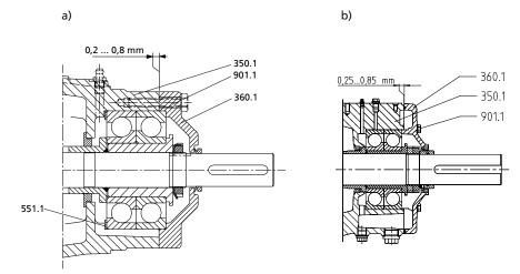
Fig. 49: Grease-lubricated bearings: a) sizes 32-200 and b) size 250
