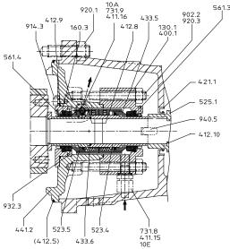
Fig. 40: Application limits of double mechanical seal in back-to-back arrangement
