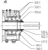
Fig. 33: Oil lubrication with lip seal: a) size 32 and b) sizes 50-65 and c) sizes 100-200 and d) size 250
