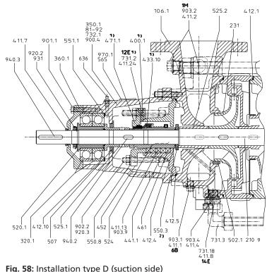
Fig. 58: Installation type D (suction side)
