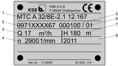
Fig. 5: Name plate (example) of Multitec
