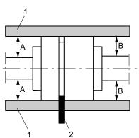
Fig. 12: Non-spacer-type coupling, checking the coupling alignment
