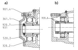
Fig. 26: Grease lubrication with lip seal: a) Multitec 32-125 and b) Multitec 150-200
