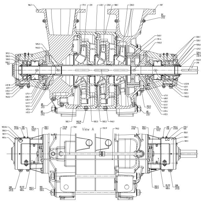
Fig. 60: Installation type C – Multitec 250
