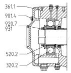
Fig. 28: Grease lubrication with lip seal: Multitec 250
