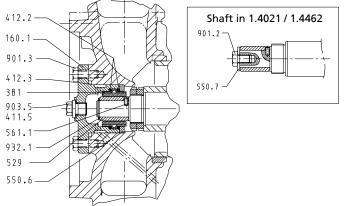
Fig. 25: Dismantling the plain bearing - radial suction nozzle
