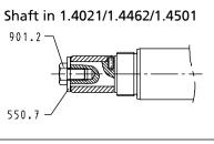
Fig. 23: Dismantling the plain bearing - axial suction nozzle
