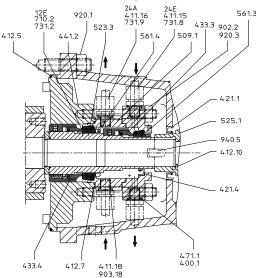
Fig. 41: Removing a mechanical seal in tandem or quench design
