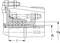
Fig. 47: Gland packing chamber
