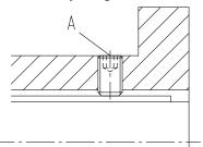
Fig. 52: Coupling hub with grub screw
