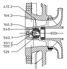
Fig. 24: Dismantling the plain bearing - axial suction nozzle
