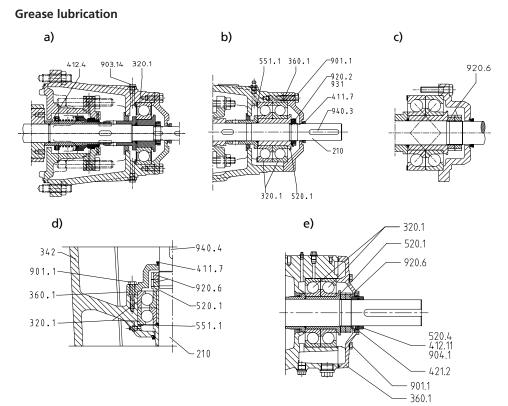
Fig. 31: Grease lubrication: a) size 32 and b) sizes 50-65 and c) sizes 100-200 and d) installation type V sizes 100-150 and e) size 250
