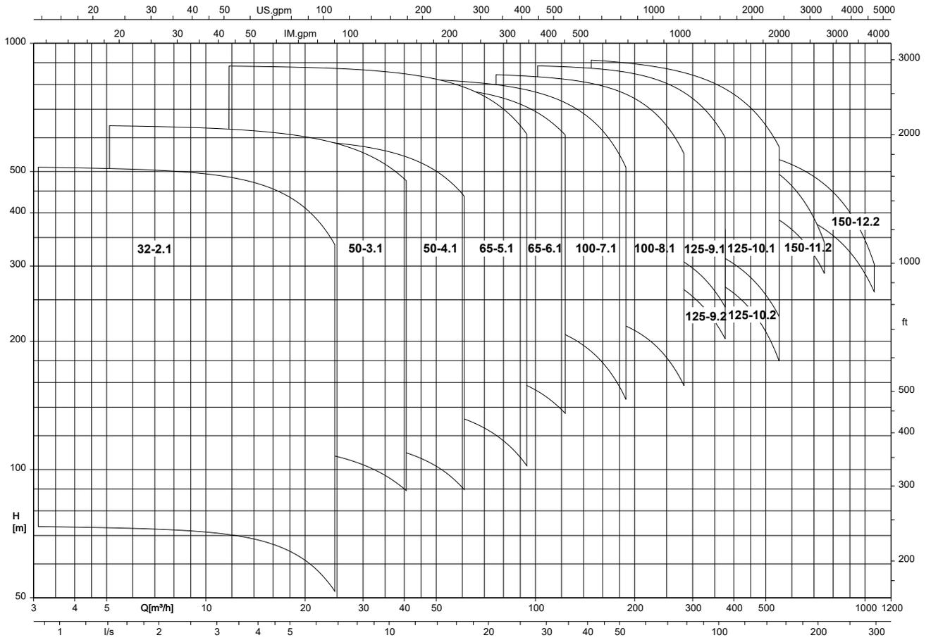
Multitec/Multitec-RO, 60 Hz, n = 1750 t/min
