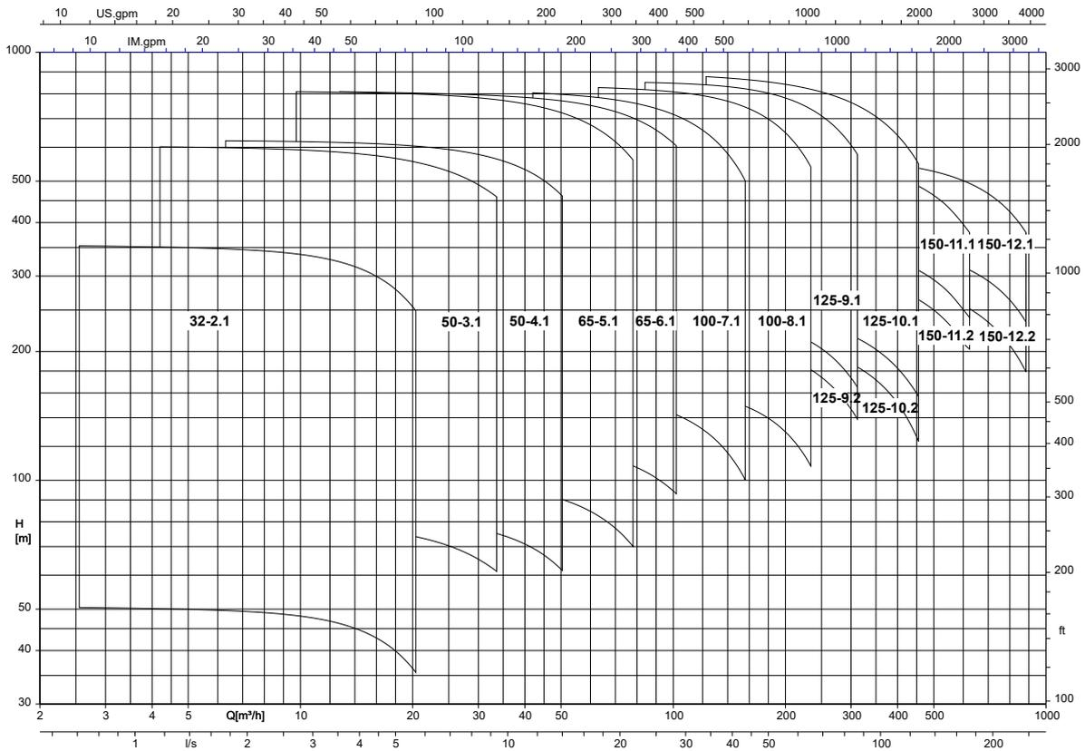
Multitec/Multitec-RO, 50 Hz, n = 1450 t/min
