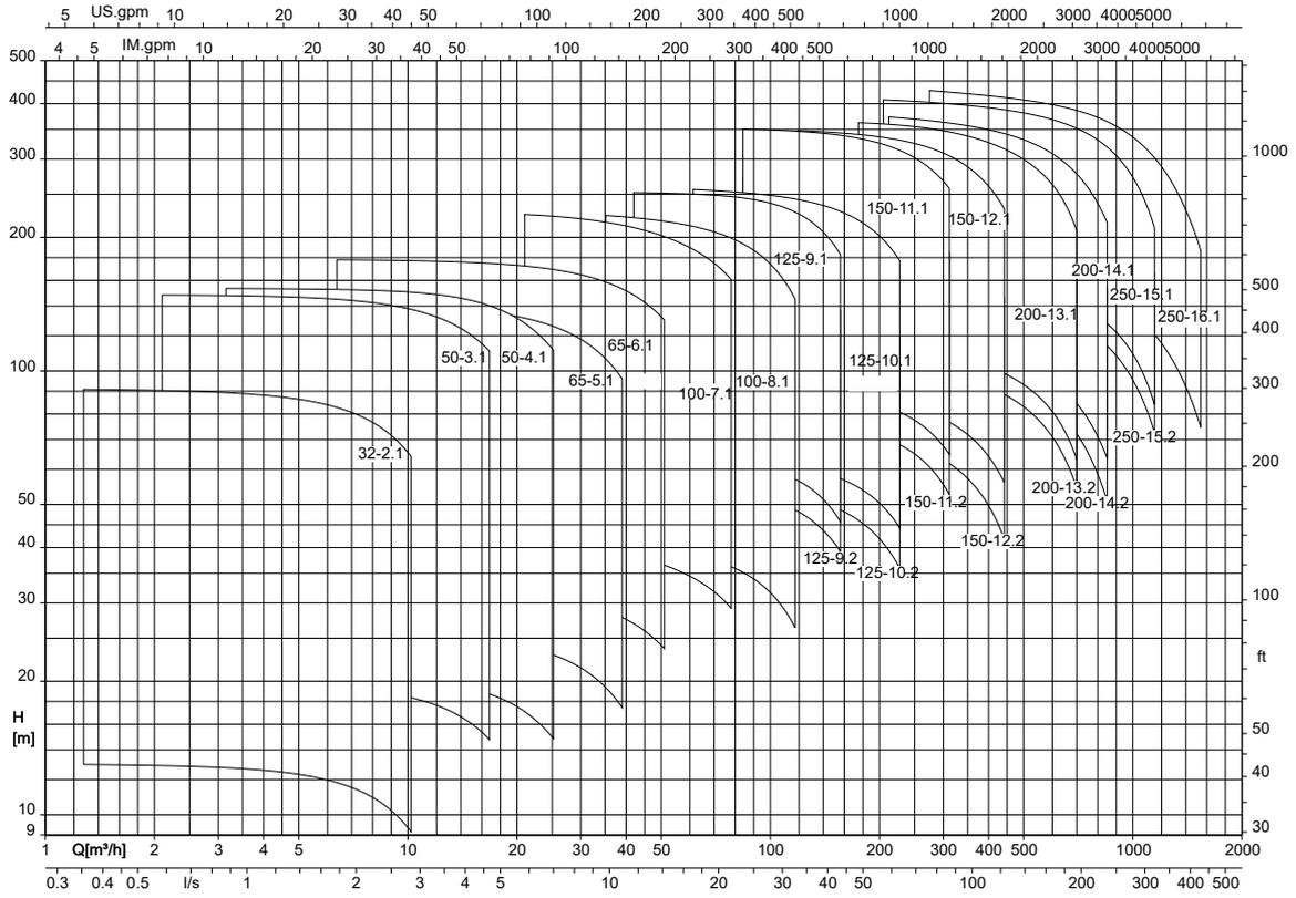
Multitec/Multitec-RO, 60 Hz, n = 3500 t/min
