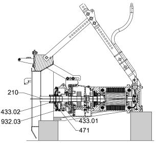
Fig. 35: Removing the mechanical seal of an Amaline 500, 600
