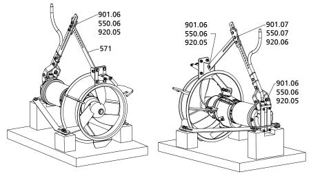
Fig. 16: Correcting the attachment point
