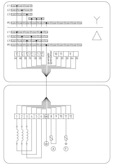
Fig. 61: Wiring diagram for Amaline 500, 600, 800 with power cables 7G4 + 5×1.5, 7G6 5×1.5 and 7G10 5×1.5
