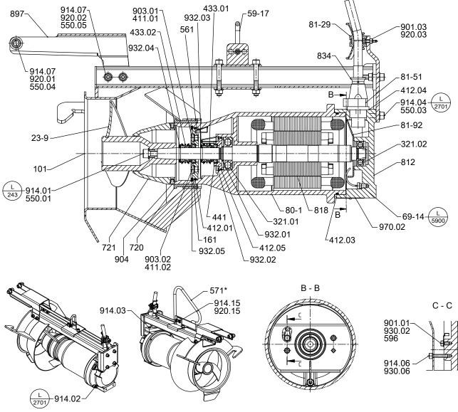
9.1.1 Amaline 200 (motors: 1 4, 2 4; motor housing made of grey cast iron)
