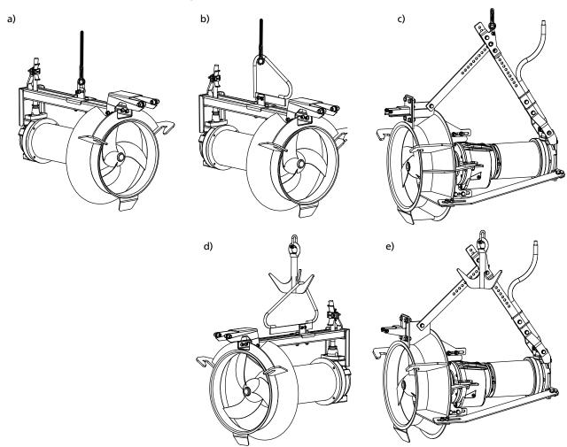
**Fig. 14:** Checking the attachment point a) Amaline 200, 300, 400 with lifting rope at shackle b) Amaline 200, 300, 400 with lifting rope at bail c) Amaline 500, 600, 800 with lifting rope at bail d) Amaline 200, 300, 400 with lifting hook at bail e) Amaline 500, 600, 800 with lifting hook at bail
