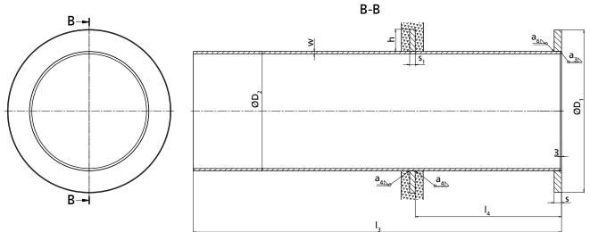
**Fig. 65:** Dimensions of the connection pipe ( $I_3$ ,  $I_4$  = order specifications provided to the manufacturer by the customer)
