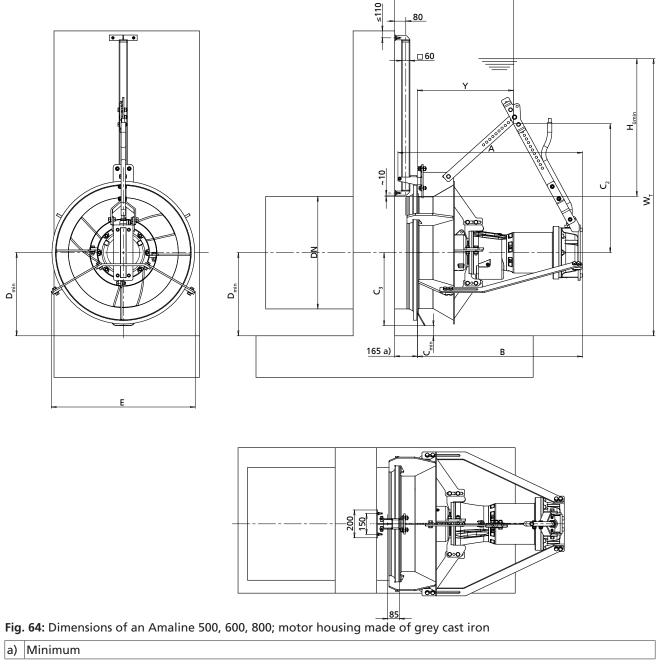
9.5.3 Amaline 500, 600, 800; motor housing made of grey cast iron
