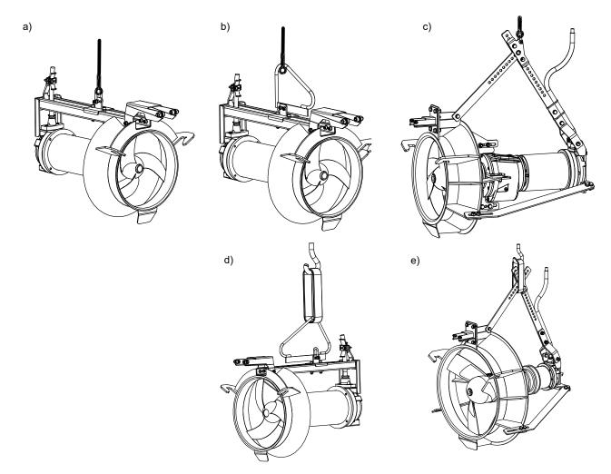
**Fig. 4:** Transporting the pump set a) Amaline 200, 300, 400 with lifting rope at shackle b) Amaline 200, 300, 400 with lifting rope at bail c) Amaline 500, 600, 800 with lifting rope at bail d) Amaline 200, 300, 400 with webbing sling at bail e) Amaline 500, 600, 800 with webbing sling at bail
