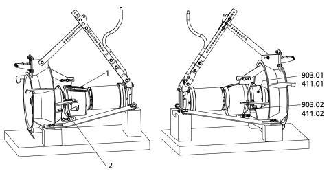
Fig. 25: Draining the lubricant of an Amaline 500, 600, 800
