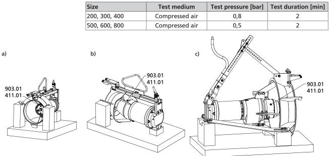
Fig. 39: Leak test a) Amaline 200, 300 with motor 0 6 or 2 6, 400 b) Amaline 300 with motor 8 6 c) Amaline 500, 600, 800
