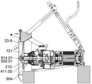
Fig. 42: Mounting the axial propeller of an Amaline 500, 600
