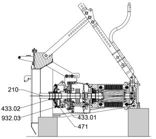
Fig. 38: Installing the mechanical seal of an Amaline 500, 600
