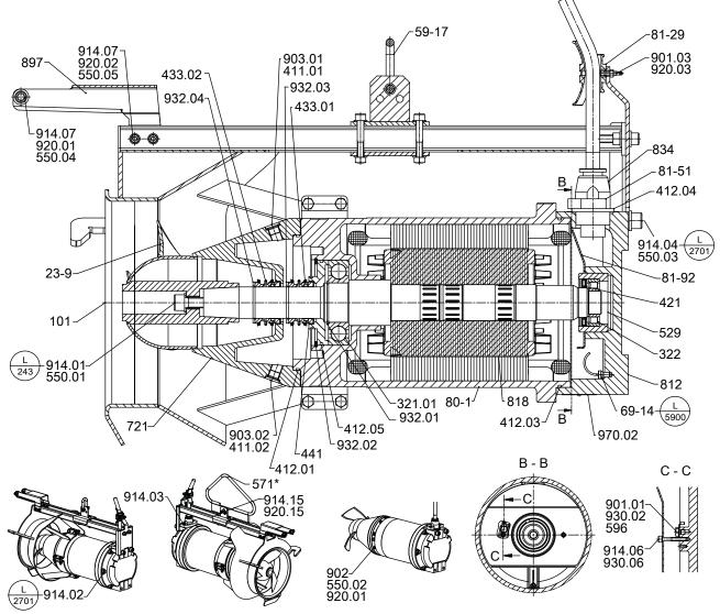
Fig. 47: General assembly drawing: a) with shackle b) with bail (optional) \*: On specific designs only
