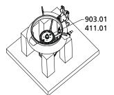
**Fig. 7:** Checking the lubricant level of an Amaline 200, 300 with motor 0 6 or 2 6, 400
