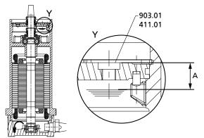
Fig. 27: Lubricant level Amaline 200, 300 with motor 0 6 or 2 6, 400
