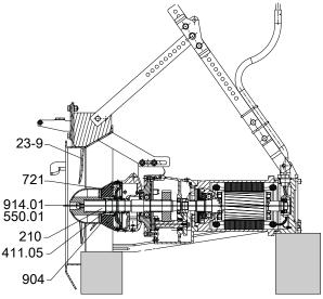
Fig. 32: Removing the axial propeller of an Amaline 500, 600
