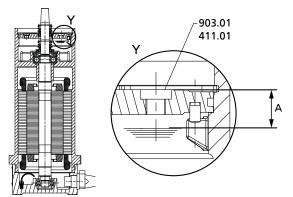
Fig. 8: Lubricant level Amaline 200, 300 with motor 0 6 or 2 6, 400
