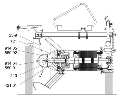
**Fig. 40:** Mounting the axial propeller of an Amaline 200, 300 with motor 0 6 or 2 6, 400
