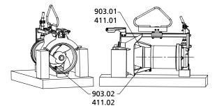
Fig. 24: Draining the lubricant of an Amaline 300 with motor 8 6
