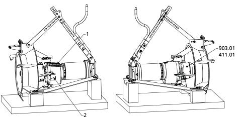
Fig. 29: Topping up the lubricant of an Amaline 500, 600, 800
