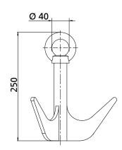
Fig. 13: Lifting hook
