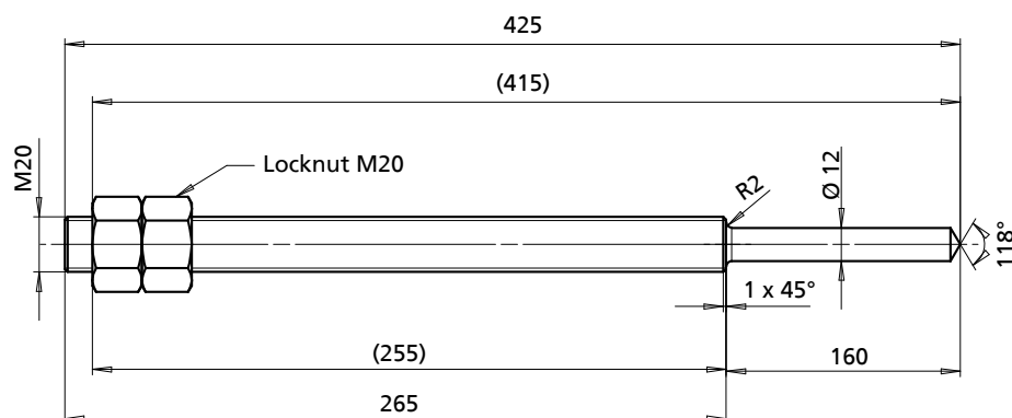
Fig. 31: Forcing screw M20 x 425
