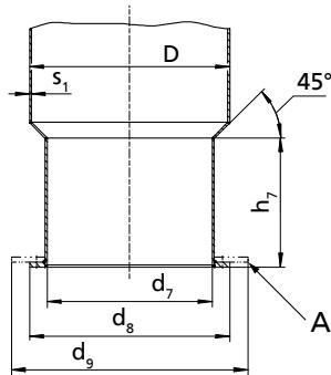
Fig. 4: Dimensions of the discharge tube
