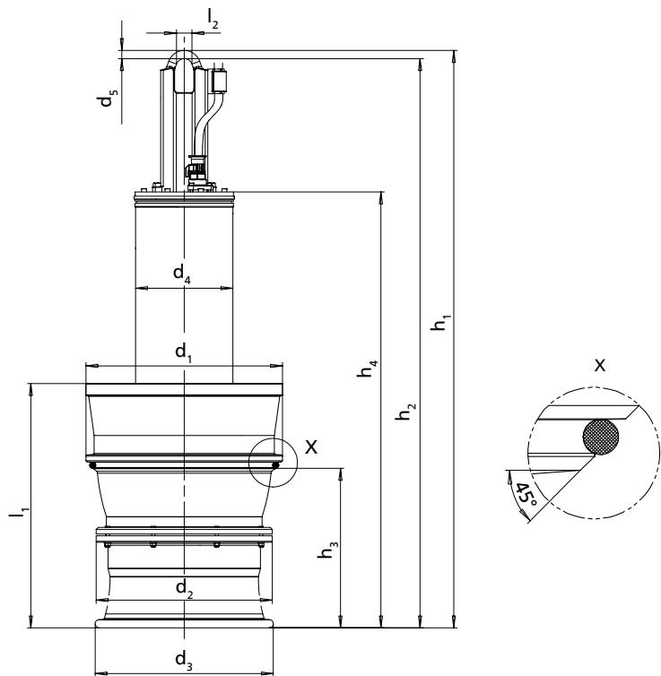
**Fig. 7:** Dimensions of the pump set
