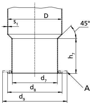
**Fig. 6:** Dimensions of the discharge tube
