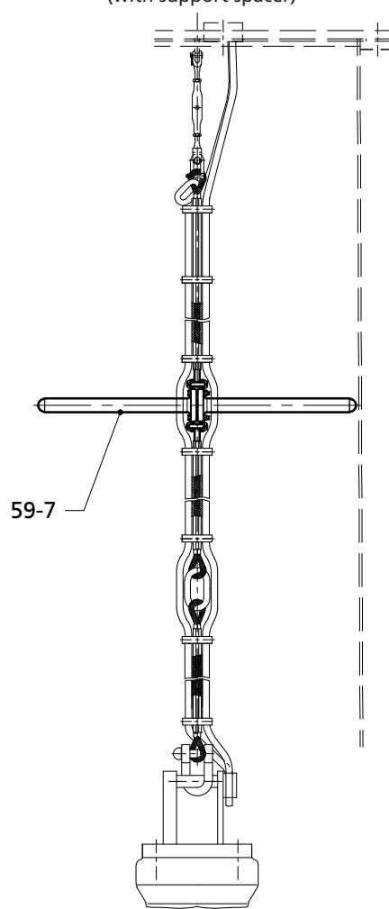
\*= The number of (intermediate) lifting rings depends on the lifting height of the lifting equipment and on the building structure. (Intermediate lifting rings are supplied as an option).
