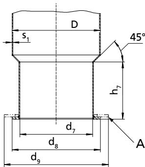
Fig. 8: Dimensions of the discharge tube
