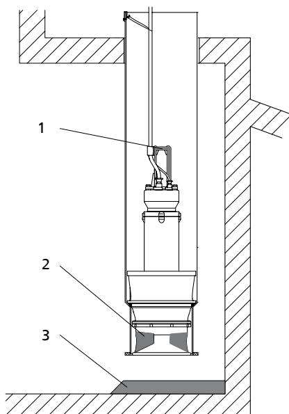
**Fig. 3:** Installation position of the pump set
