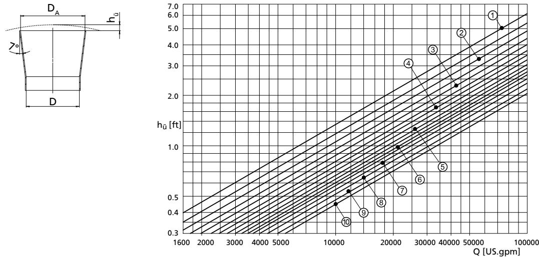
Illustration of the overflow head  $h_u$       Loss diagram
