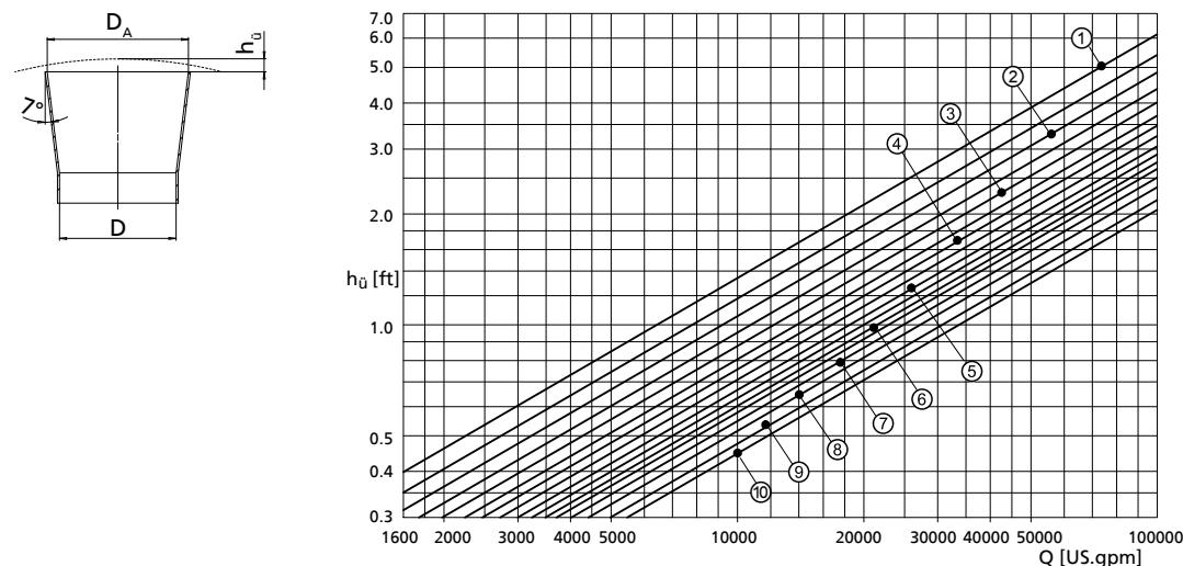
Illustration of the overflow loss diagram
