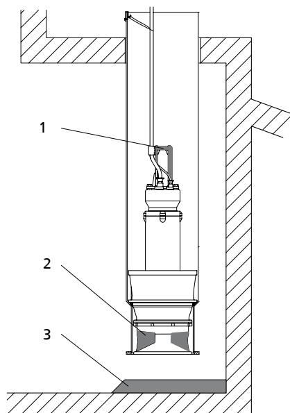
**Fig. 1:** Installation position of the pump set
