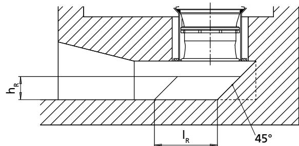
Fig. 4: Flow-straightening vane for covered intake chamber
