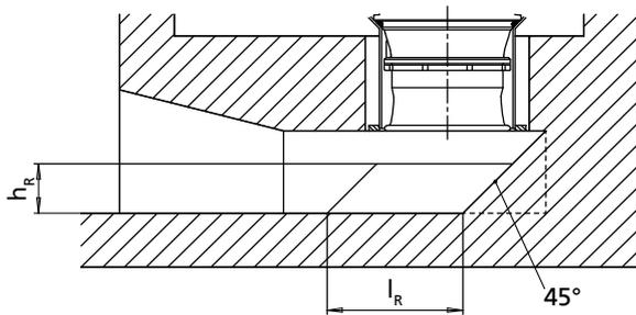
Fig. 2: Flow-straightening vane for covered intake chamber
