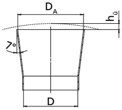
Illustration of the overflow head  $h_{\bar{u}}$
