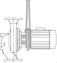
Abb. 1: Pumpenaggregat transportieren
