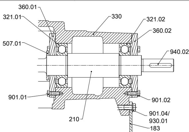
III. 29: Version support de palier WS 50, WS 60 et WS 60.1
