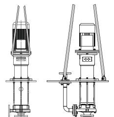
Fig. 1: Transporting the pump set without/with cover plate up to motor size 160
