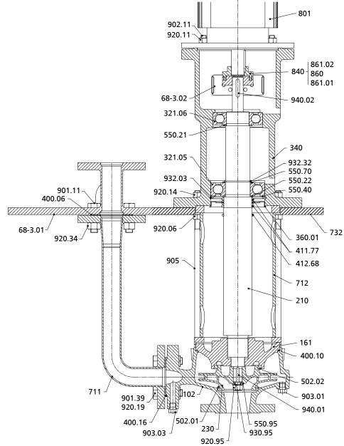
Fig. 12: General assembly drawing Etanorm V, design D
