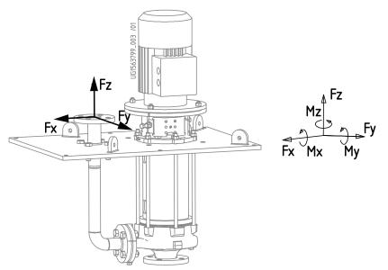
Fig. 8: Forces and moments at the pump nozzles
