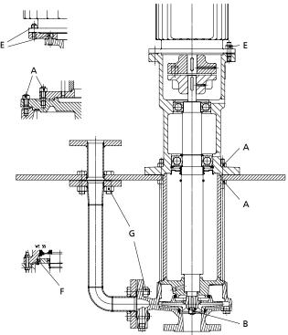
Fig. 11: Tightening points
