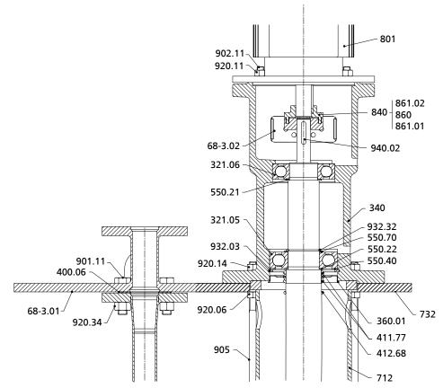
Fig. 6: Fastening the pump with motor
