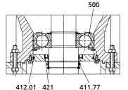
Fig. 10: Shaft seal for shaft unit 55
