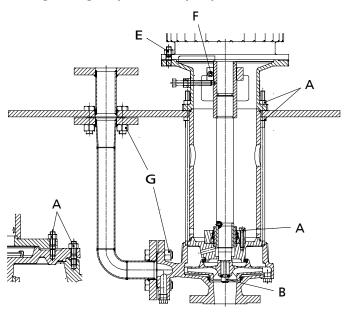
Fig. 12: Tightening points
