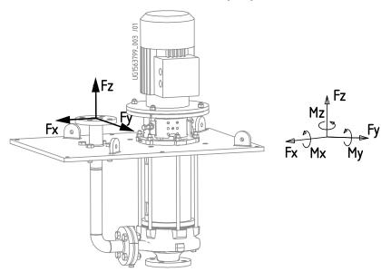
Fig. 11: Forces and moments at the pump nozzles
