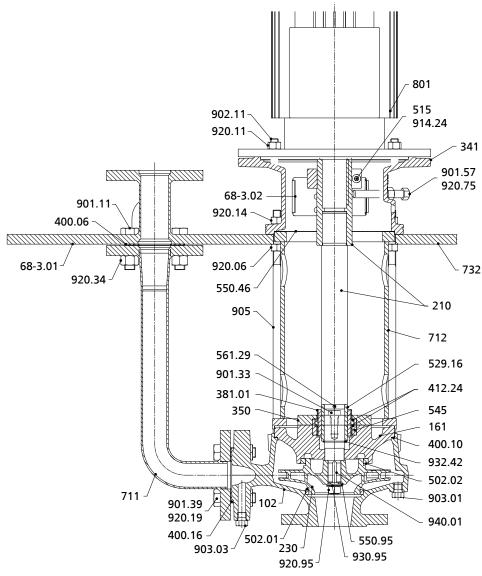
Fig. 13: General assembly drawing Etanorm V, design W
