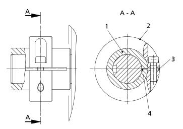
Fig. 10: Position of the locking ring
