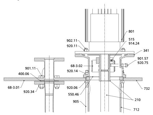
Fig. 8: Fastening the pump with motor
