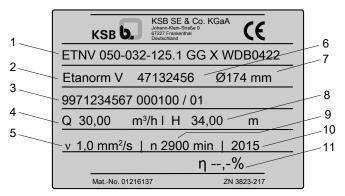
Fig. 5: Name plate (example) Etanorm V - design W
