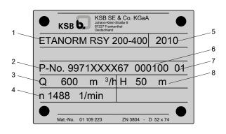
Fig. 5: Name plate (example) Etanorm-RSY
