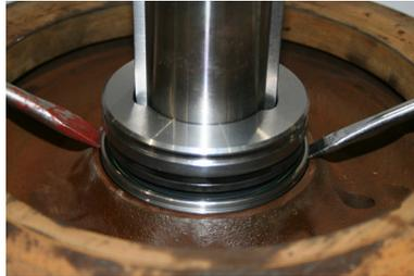
**Fig. 16:** Prising out the mechanical seal using pry bars
