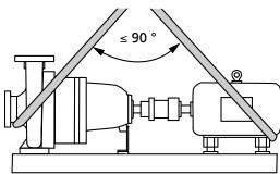
Fig. 3: Transporting the pump set
