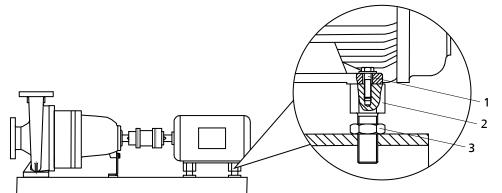
Fig. 13: Levelling the pump set with adjusting screws
