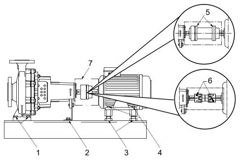
Fig. 24: Tightening points at the pump set
