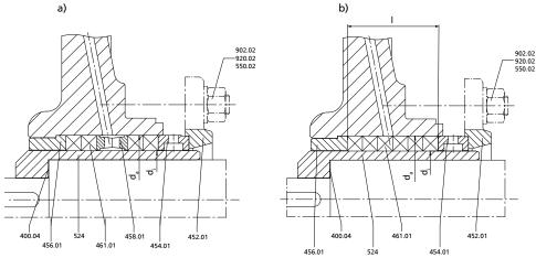
Fig. 21: Packing the gland a) with lantern ring and b) without lantern ring
