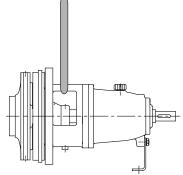
Fig. 1: Transporting the back pull-out unit
