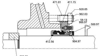
└─ 509.95 Fig. 15: Removing the KSB cartridge seal (4ES)
