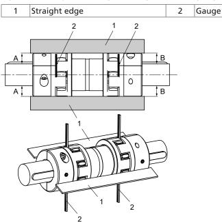
Fig. 12: Double Cardan spacer-type coupling, checking the coupling alignment
