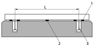
Fig. 7: Fitting the shims
