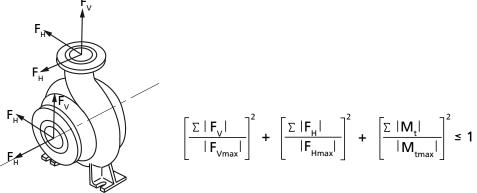
Fig. 9: Forces and moments at the pump nozzles
