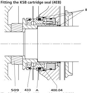
Fig. 20: Fitting the KSB cartridge seal (4EB)
