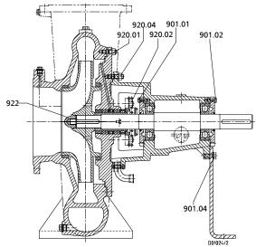
Fig. 23: Tightening points at the pump
